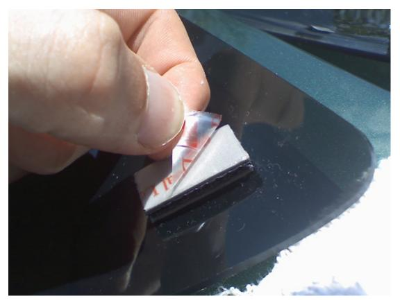
4. If the headlight covers aren't lined up the way you want them to be, quickly remove them because the double sided tape will quickly bond after a few seconds. You can then try again to match it up correctly.
