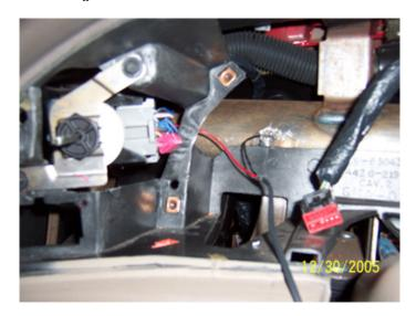
11. Now that the electrical portion is complete, go ahead and reconnect your battery. This will allow you to test the new gauges to make sure that your electrical connections are correct. Once you are satisfied that the gauges operate to your satisfaction, button everything back up by reversing steps 5 through 1. The headlight knob will just slide back on; there is no need to fiddle with the clip anymore. Enjoy your new gauges!
