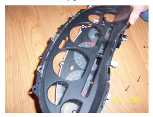
8. Some gauge inserts will allow you to slip the insert over the existing overlay. An easy way to tell if this is the case is to look at the holes in the insert where the needles will go. If they are large enough to accommodate the black circular needle mount, simply slip the insert over the needles and onto the cluster. Be careful not to break or over-stress a needle during this step; an additional set of hands will be useful.
