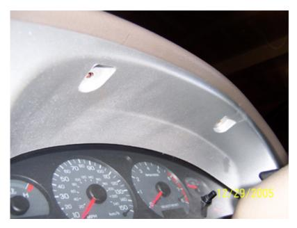
4. After the dash panel is removed, this is what your dash will look like. There are four T-15 screws, two on each side, of the gauge cluster which secure the cluster to the dash. Remove these screws.
