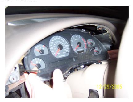
6. Here is what your dash will look like after the gauge cluster is removed. Note the two connectors referenced in step 5.
