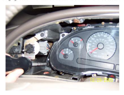
5. Lift the gauge cluster gently out of the dash. The cluster is additionally restrained by two electrical connectors which connect the gauge cluster to the PCM. They have a push clip in the middle which, when pressed, will allow the connector to be removed from the gauge cluster. Once the cluster is free of both connectors, remove it from the dash.
