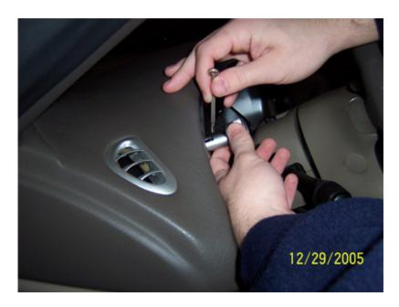
3. Once the headlight knob is off, use the T-15 Torx bit to remove the two screws holding the dash panel to the dash. Once they are removed, the panel will pull outwards with moderate effort. Note that the panel is additionally secured with clips and pins behind the dash, so be careful to only pull straight outwards to avoid bending or breaking them.
