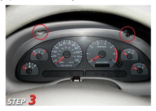
4. Remove the gauge cluster from the dash. Begin by removing the four T-15 (or Phillips head) screws securing it to the dash. Gently pull it away from the dash and release the two clips connecting it to the electrical system. The picture below illustrates the 2 connectors you will have to release for the gauge cluster to be removed from the vehicle.
