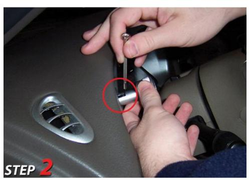
3. Remove the 2 screws holding the dash panel to the dash with the T-15 Torx bit. Once removed, the entire panel can be removed by pulling straight outward with gentle but firm pressure, which will release the clips and pins also securing it in place at the bottom and around the steering column.
