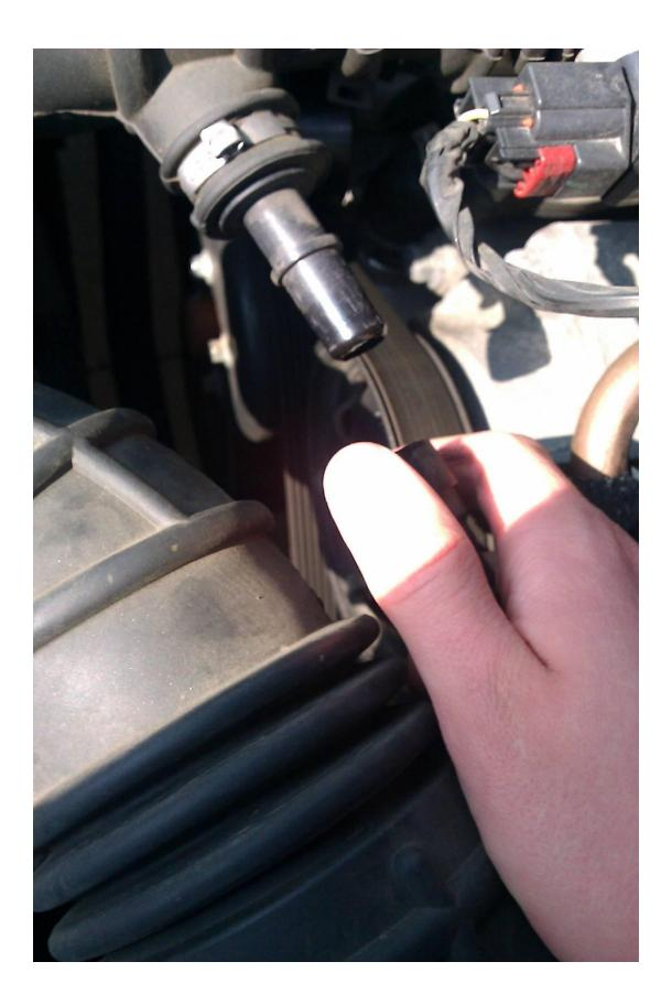
2. Using the screw driver, unscrew the clamps of the stock intake hose. (there is one that holds the hose onto the throttle body and one that holds the hose onto the 3. Remove stock hose and set aside. It should look like this after you remove the stock intake hose:
