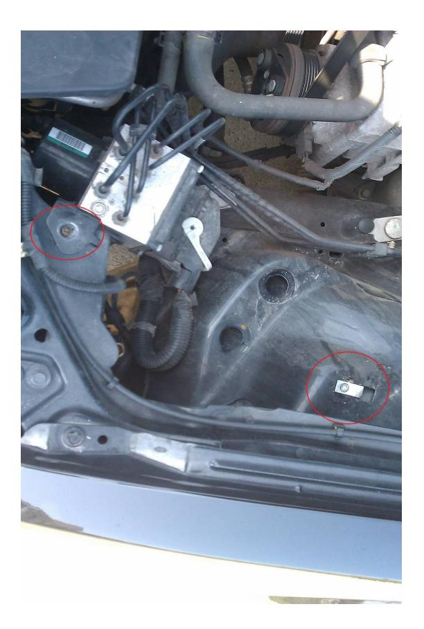
5. Align the holes in the heat shield up with these bolt holes and secure it down. It will look like this:
