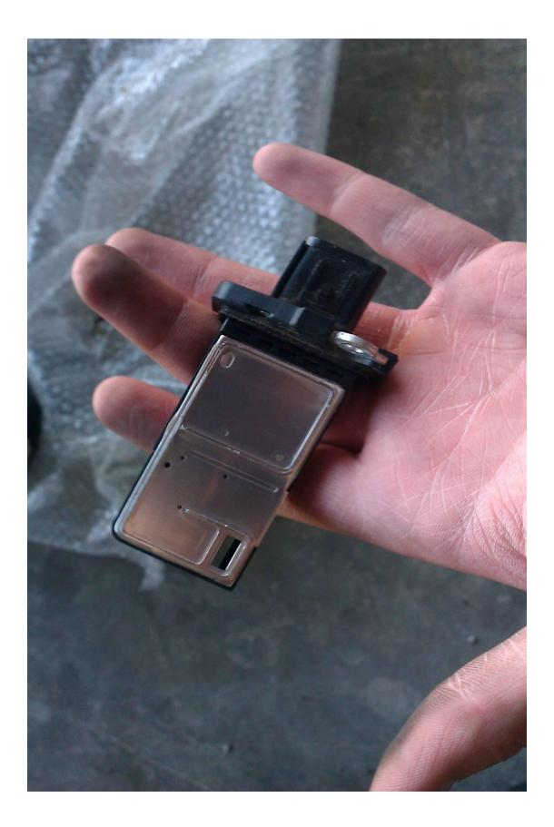
9. Place the MAFS into the Cold Air Intake's piping (the mounting area will look nearly identical to that of the factory air box. This action will utilize the same screws with T15 Torx heads.)
