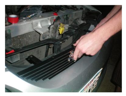
6. Slide the mounting hardware and fasteners that came with the grille into the lined up holes and hand tighten. I didn't bother using tools for this part; hand tightening was all it needed.
