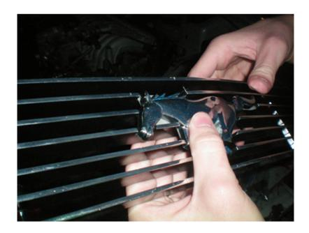
5. Place the grille in its designated spot on the car, lining it up with the pre-cut holes that Ford left for us, but no grille for some reason.
