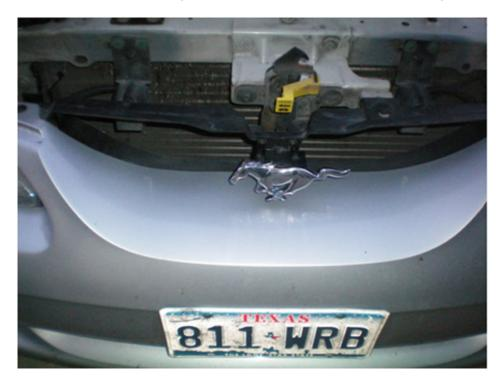
2. Using you Torx screw driver, unscrew the Torx screws that secure the pony bracket to the car.
