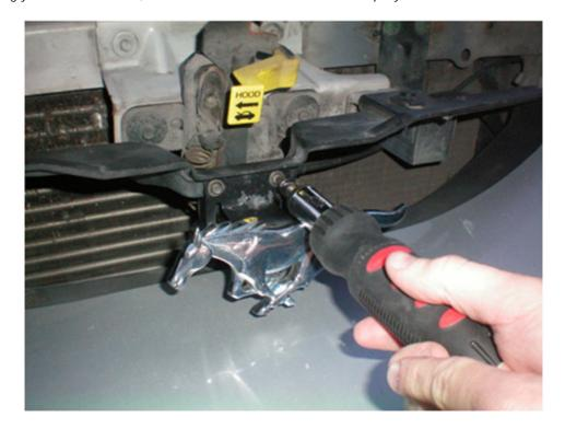
3. Pull the pony emblem off of the bracket with your fingers. This should be pretty easy to do. You will no longer need the bracket, just the emblem. Using the wire cutters, cut off the post on the back of the pony emblem that had previous connected it to the bracket. This should give the pony emblem's back side a flat surface that will make the next steps much easier. There should be four different posts to cut off.
