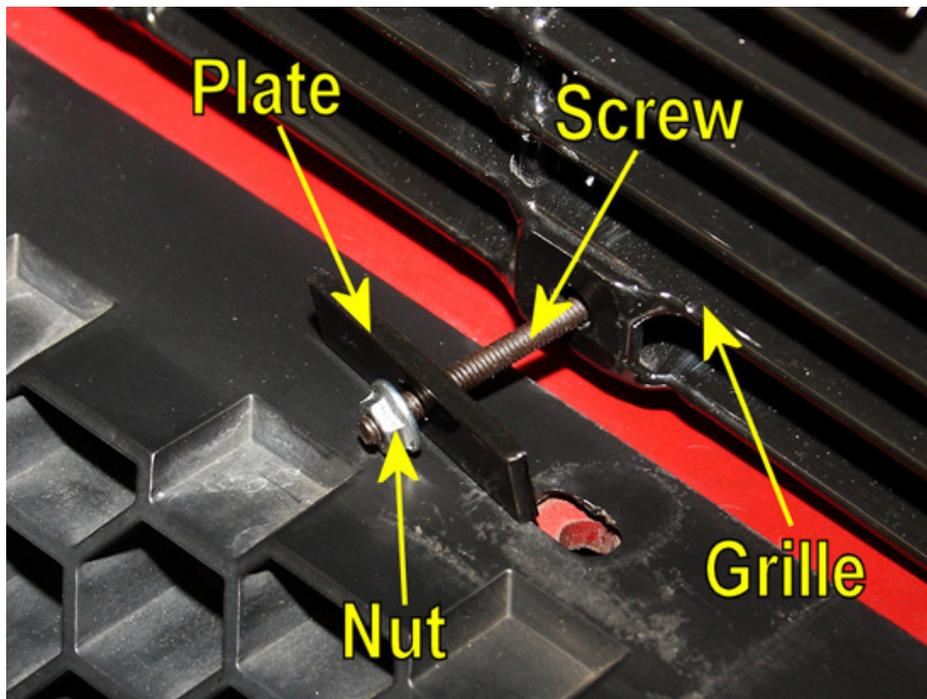
6. Once the grille is positioned against the front of the factory grille, install the supplied hardware to hold it into place. All you need to use to tighten the screws down, from the front, is a Phillips head screwdriver. You can easily prevent the nut on the backside of the grille from turning with your fingers. Once completed, reinstall the radiator cover and factory fasteners you removed earlier.
