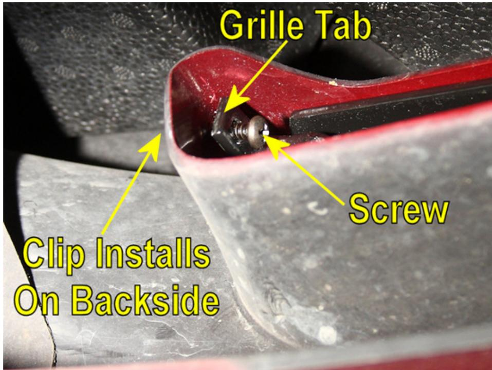
12. To tighten the screws, a long screwdriver passed through the front of the grille is an easier method than trying to tighten the screws up from the backside of the bumper cover.
