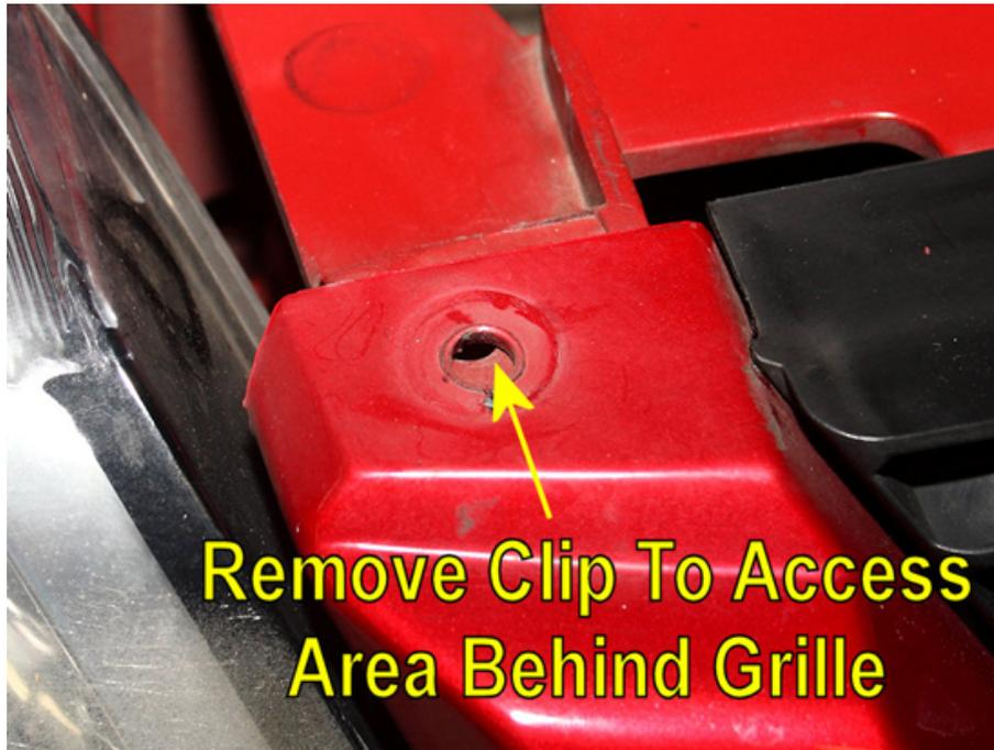
5. The Billet Grille uses a screw, nut, and metal plate to secure itself to the factory grille. The factory grille will be sandwiched between the plate and the billet grille.
