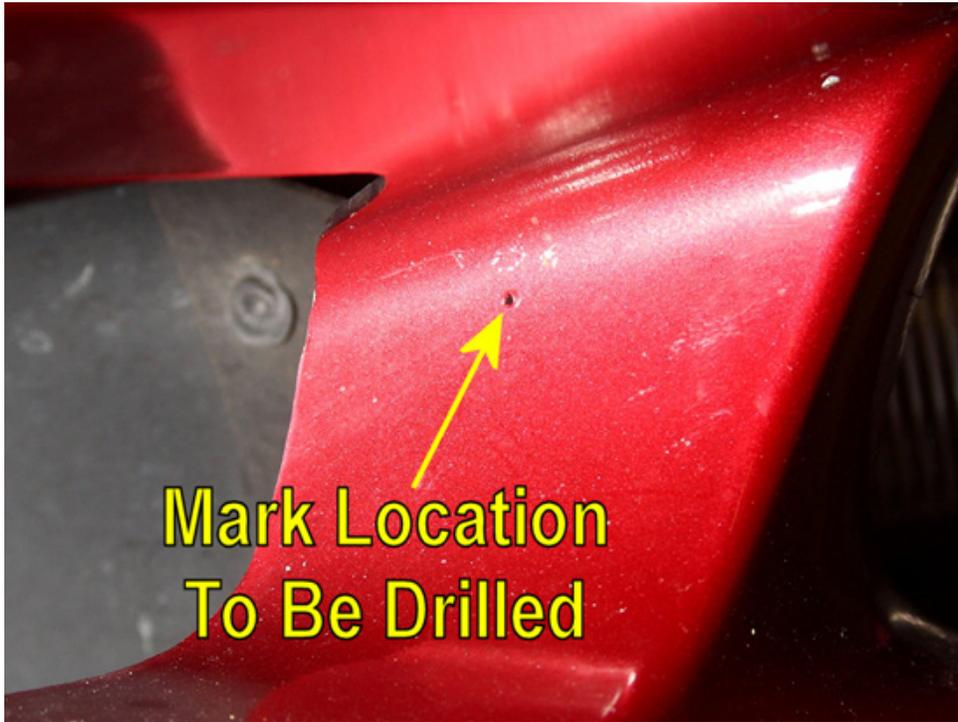
10. When installing, the screws will pass through the tab on the grille, then through the bumper cover, and then be held in place by the supplied metal clips.
