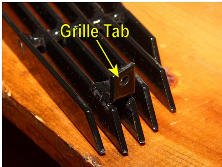
9. Position the grill in place, and then mark the spot for the holes you'll drill. I used a punch, but you could just as easily use a Sharpie permanent marker or similar marking tool. Then use a drill bit, an 1/8 inch bit works well, to drill holes for the screws.
