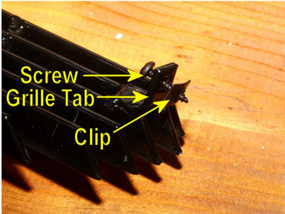
11. Place the grille into the car's bumper cover, and thread the screws on each end down into the metal clips. The clips will go on the backside of the bumper cover. This step is easiest accomplished while under the car, which is why the car was raised earlier.
