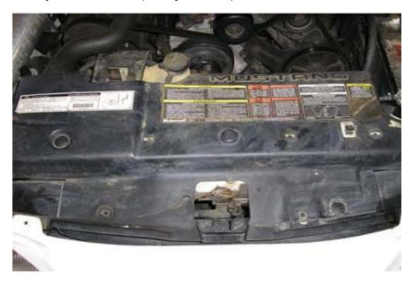
2. To remove the pony and its bracket, simply unscrew the 2 Philips head screws that are holding it to the vehicle.
