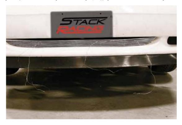
5. Twist the wires until the grille is held securely in place. Trim excess wire with the wire cutters and wrap the ends of the wires in electrical tape to prevent scratching your paint.
