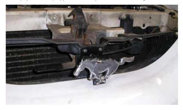
3. Set your pony and bracket face-down on a clean, dry surface. To separate the pony from the bracket, use a flathead screwdriver to pry the round retainer-style clips off the back of the pony off the plastic prongs. If it will not easily release, you may also use a needle nose pliers to twist, pull, and gently break the 4 plastic prongs that are held onto the back of the bracket with the round retainer-style clips. This will allow you to separate your stock pony from the bracket.
