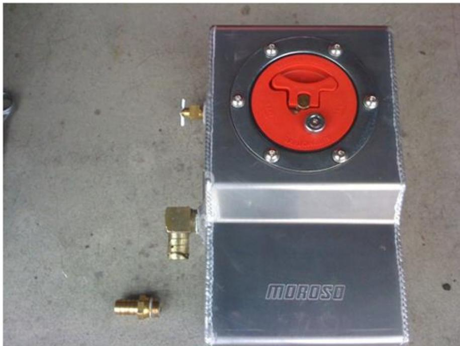
11. The lower feed fitting on the back of the new tank may need to be clocked slightly to allow an easier connection of the lower feed tube. Using an adjustable monkey wrench, I rotated the fitting about 45 degrees counter clockwise to match the angle of the old tanks clocked fitting position. If this step is not applicable to your setup, continue to step 12.
