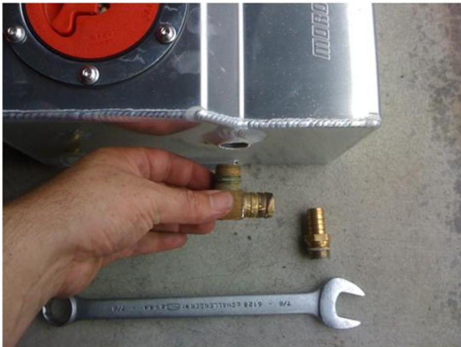
9. Before installing the old brass fitting into your new tank, make sure to use some type of anti cease. I prefer the silicone tape type, make sure to wrap all the threads. I would also recommend cleaning the old fitting first with a wire brush and brass polish to remove and tarnish or debris.
