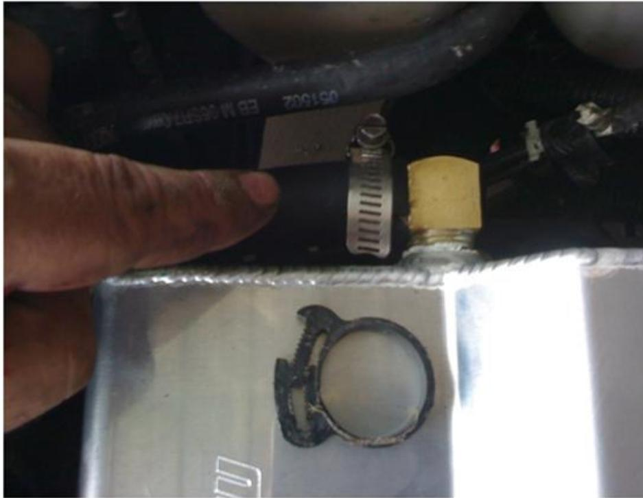
14. Reinstall the tank hold down clamp wedge by reversing step 4. Make sure to position the tank squarely on the battery platform before tightening down. Also, reconnect all wires and any other obstructions that were removed in step 2.
