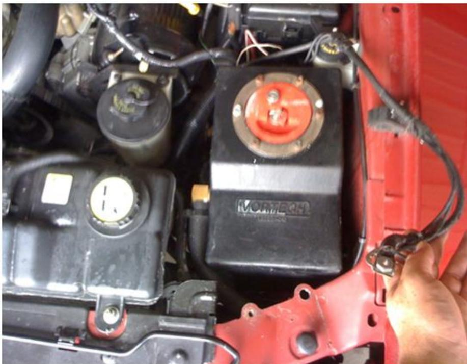
3. Drain water/coolant from the old supercharger reservoir tank. Near the back and bottom corner there is a brass twist valve. Twist valve open and drain into a catch bucket or container placed directly underneath. Location may slightly vary depending on your supercharger brand.
