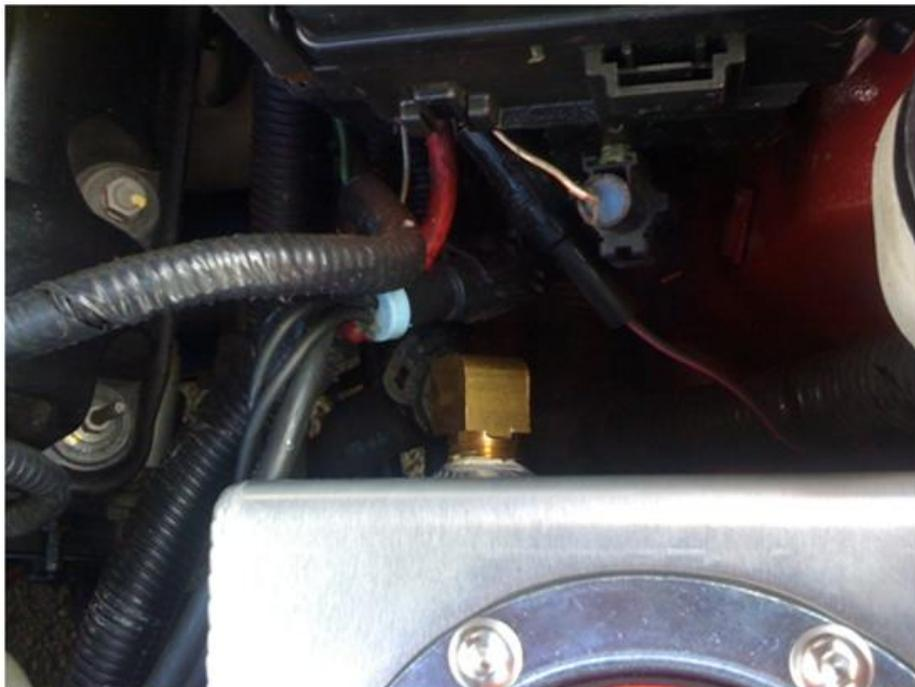
13. Now that the lower hose is connected, you can connect the upper return hose to the upper fitting. Note that I decided to use steel hose clamps vice the plastic ones that came with the Vortech kit. This is just a preference, but is not necessary for installation.
