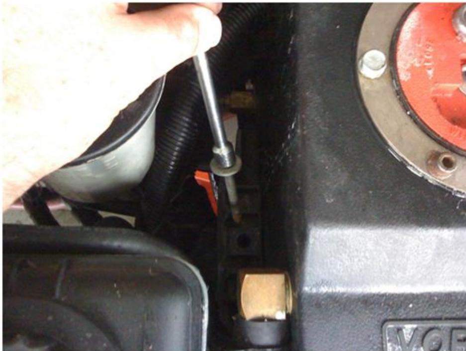
5. First disconnect the upper return hose. There is a small plastic zip clamp holding on the hoses to the fittings. Use flathead screwdriver to pry apart the zip clamp to allow the hose to be pulled off. If hose is stubborn to come off, gently use your flathead screw driver to assist in prying it off as you pull, being careful not to tear the hose.
