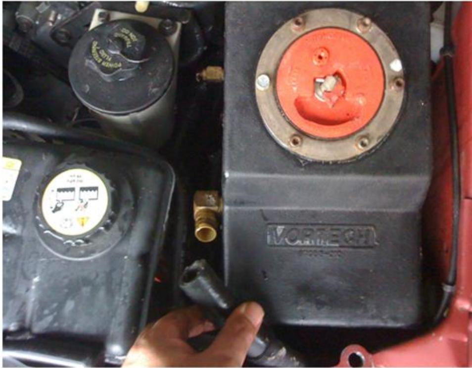
6. Repeat step 5 for the bottom feed hose. Seeing how you have already removed the upper return hose and the tank hold down clamp, the tank can easily be lifted out to allow easier access to disconnect the bottom feed hose.
