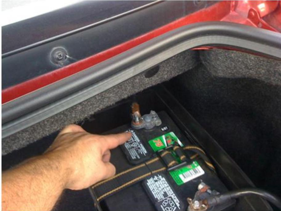
2. Start by removing any and all obstructions that may be in the way of the removal and installation process of the supercharger tank. In this case, it was just several grounding wires. Remove bolt with a 5/32" socket and gently pull wires aside and out of the way.
