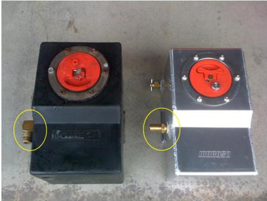
8. Using a 7/8 inch wrench turning counter clockwise, remove the upper brass return fittings from the old and new tanks. Below is a comparison of the two fittings.
