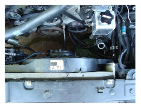
7. Place the Moroso expansion tank in place of the factory tank reusing the factory 10mm nuts.
