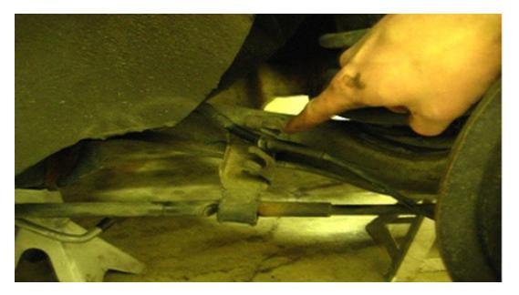
9. Pick one side of the car to start with first and raise the jack, with the small piece of wood on the jacking cup, so that the bottom of the control arm is supported but not lifting the car.
