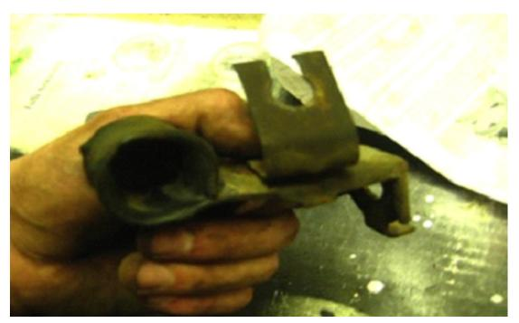
16. Slide the parking brake cable back through the bracket, then slide the parking brake back through the slot on the bottom of the control arm, and place the e-clip back into position. Finally use the pliers to attach the parking brake back to the caliper.
