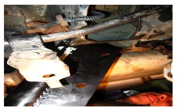
18. Place the jack back under control arm and place the spring on the spring perch, raise the jack slowly and align the spring with the upper cup and the rear bushing with the axle brackets. Place the bolt trough and torque to 85 foot pounds.
