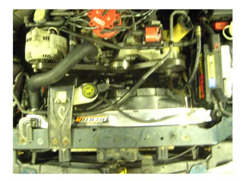
13. Secure the radiator shroud back onto the car with the 8 plastic push pins that were removed in the beginning.
