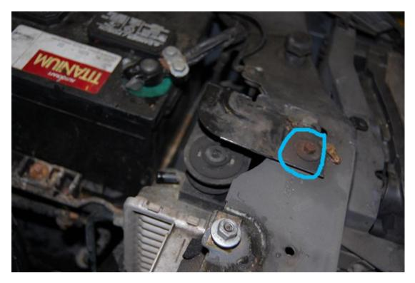
4. Remove the 8mm bolt, which holds the radiator mount to the radiator support and set the mounts aside. Then disconnect and remove the upper radiator hose. You do not have to remove it from the thermostat housing, but it does make things easier as it won't be in the way when putting in the new radiator.
