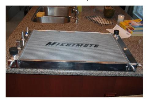
9. After unpacking the radiator, remove the drain cock, inlet/outlet caps, and transmission line plugs. Once removed, place the radiator in the car, making sure the dowels on the bottom go into the rubber mounts. Reach under the right/passenger side of the car and reinstall the drain cock.
