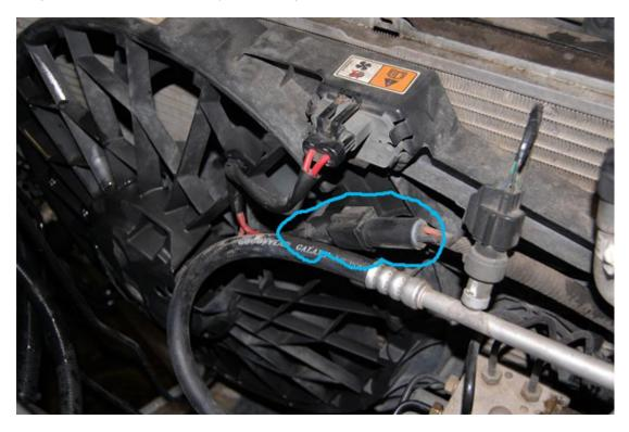
5. Unplug the fan. This is where the miniature pick comes in handy to lift up the tabs on the plug. There is a tab on the top and bottom side.
