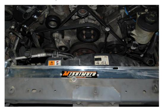
11. Slide in the fan assembly, making sure it slips into its mounting slots/tabs, and bolt it to the radiator using the two, 8mm bolts you previously removed. Reconnect the lower radiator hose, fan wiring/plug. Install the upper radiator mounts and the radiator cover in the same fashion you removed them.
