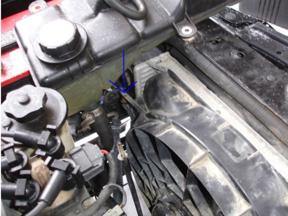
7. Next you unclip the connector from the radiator fan motor. After that, the fan will be loose. Move it slightly towards the driver side of the car, and pull up on the passenger side and the whole fan should come out no problem.
