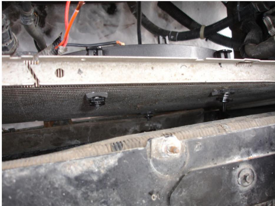
11. After installing the radiator fan, you can bolt the radiator mounts back into place. Next, you can do the wiring for the new fan. There are many different ways you can do this. One way is to find the orange and blue wire and connect it to the blue wire on the fan, and then connect the black wire from the harness to the black wire on the fan. There will be a red and orange wire left. You can tape this one off as it will not be needed.
