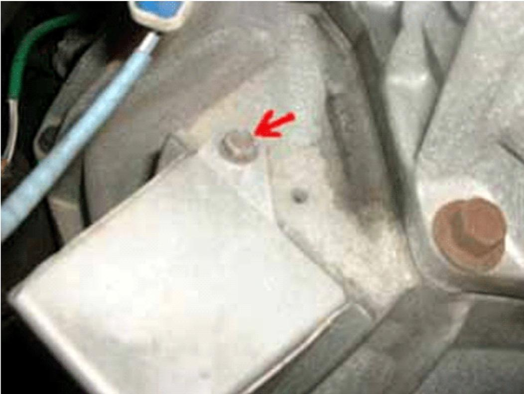
6. There is one 3/8" bolt holding this piece on (Indicated with the red arrow). Remove the bolt and slide off the cover. Watch out for the dust in there, it is a carcinogen. A dust mask is recommended; do not blow on the components inside the cover.
