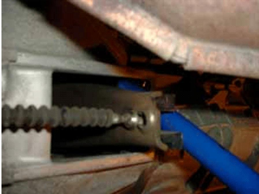
8. After the cable has been disconnected at the bellhousing, lower the car if you're using jack stands. The rest of the work will take place under the hood or under the dash.
