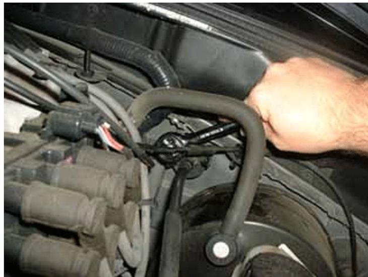
11. After removing the two bolts, pull the clutch cable out from the firewall. Be careful not to crimp the clutch cable unless you plan on replacing it with an adjustable one.
