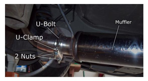
17. Put a U-Clamp around where the muffler and inlet pipes meet.
