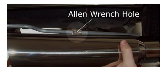
15. Slide the band clamp over the muffler tip and begin to tighten. Make sure the tip doesn't move any while tightening. If it does, just loosen the clamp (or the threaded lock), reposition, and re-tighten.
