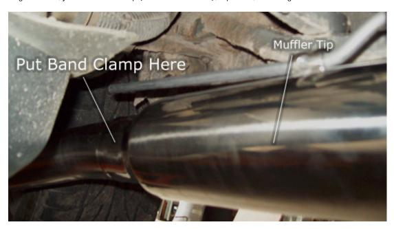
16. Take your U-Clamps and place them around where the extension pipe and muffler meet. Go ahead and put the nuts on but do not tighten them yet. It's always best to do the tightening last after you make sure everything looks well and the clearance is set.
