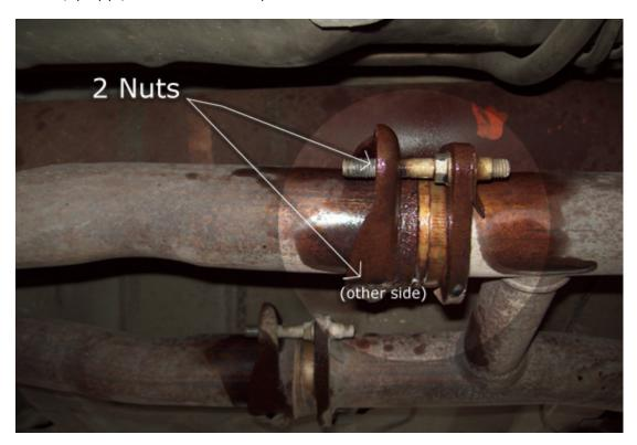
3. Find the muffler and get your sawzall ready. Right behind the muffler (in between the muffler and hanger), we will need to cut through the pipe. This prevents us from having to drop the axle to remove the mufflers. You may end up breaking a few blades, so have a couple of them handy.
