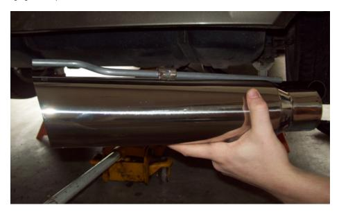
13. Put the muffler clamp on the extension pipe so that you do not forget to do this. Now slide your muffler tip onto the extension pipe as far back as it can go, and slide the rod into the hanger. Once the hanger rod is in it's place, you can slide the tip to where you would like. Note: Magnaflow recommends atleast a 1/2" gap between the muffler tip and bumper to prevent any heat-related damage.
