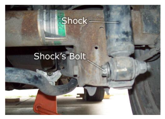
8. Once the bolt is removed, pull the shock towards the rear of the car so that it is not held in place anymore. Gently lower the jack (tire) down about 2-4 inches. This should give you enough room to slide the extension pipe in very easily. Now simply raise the axle back to its original height and screw in the bolt to hold the shock (as you are putting the bolt in, raise/lower the axle to make sure the bolt is going in straight and not at an angle).
