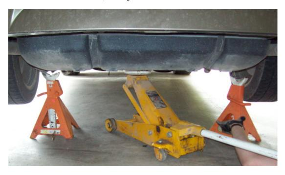
2. Underneath the middle of the car, you will find where the cat-back and mid-pipes connect. Spray some lubricant on the 2 nuts (2 per pipe) and unscrew them. Keep these nuts! You will need to reuse them.
