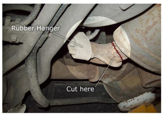
4. Now we need to pull out the muffler. Spray the rubber hangers with lubricant, then pull out the muffler from the mid-pipe so that the muffler is hanging down. After that, you pull the hanger rod out of the rubber hanger.
