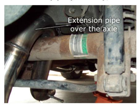
9. Now that the extension pipe is in place, we need to hang it up. Like before, lubricant helps tremendously. Push the hanger rod, located on the extension pipe, through the rubber hanger shown in the image below.
