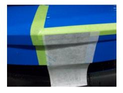
**Step 5:**Leaving the tape on peel back the vinyl out of the way on the bottom .
