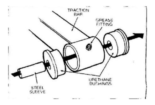
2. Apply lubricant (supplied) to polyurethane bushings and steel sleeves, then install into eyelet ends as shown.
