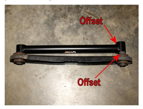
11. Now, it's time to examine the hardware that comes with the suspension arms. There are four steel sleeves, two long ones and two shorter ones. The short ones are for the front, the longer ones for the rear.
