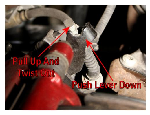
6. Pass the parking brake cable through the factory lower control arm.
