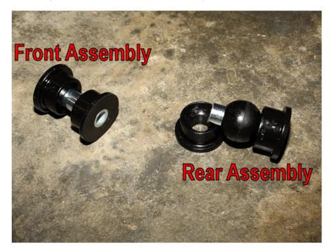
14. Once you know how to assemble the bushings, you'll want to grease them with the supplied grease. Grease the outer portion of the sleeves, and the inner portions of the bushings. Also grease the outside of the bushings with the exception of the bottom that they're resting on in the picture below. The bottom of the bushing will face the suspension mounts on the car, and doesn't really need any lubrication.
