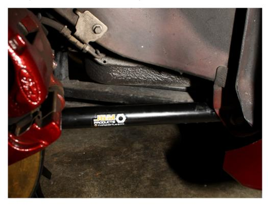
The parking brake cable will simply rest on the suspension arm, once you reconnect it to the assembly. You can use a wire tie to hold it in place if you prefer, but it's not necessary. 18.
