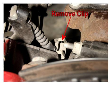
4. Now locate the cable, cable end, and brake lever, as shown in the picture below. They are just above the clip you removed.
