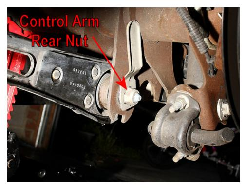
10. When removing the lower suspension arms, make sure to keep it oriented correctly, or note which end is the front and which is the back. The two ends are offset differently, and you must make sure correctly install the new suspension arm in regards to its offset. The rear of the new arm is wider, to match the larger width of the stock arm. This area is offset as well, just like the stock arm. The larger offset should face the middle of the car when it's installed.
