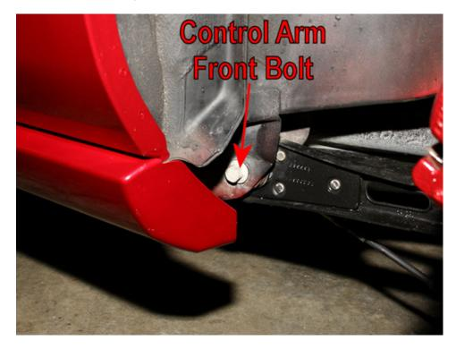
8. Once the front bolt removed, you'll want to do the same with the rear bolt. Again, an 18mm socket and socket wrench needs to be used.
