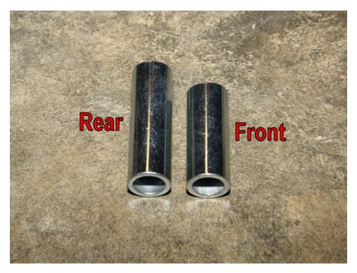
12. You'll also find two different style bushings. Some with a concave face that curves inward, while the others utilize a flat face. The flat-faced bushings are for the front, while the curved ones fit the rear of the suspension arm.
