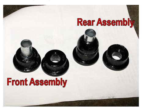
15. You'll also want to apply some grease to the inside of the control arm. Once that's done, press the bushing assembly into place from one side of the control arm. Before pushing the other side's bushing into place, I found it's best to push the steel sleeve halfway out of the installed bushing. This helps to allow air between the bushings to escape, and helps the remaining bushing to seat easier. Once the bushing is in place, you can push the steel sleeve in fully.
