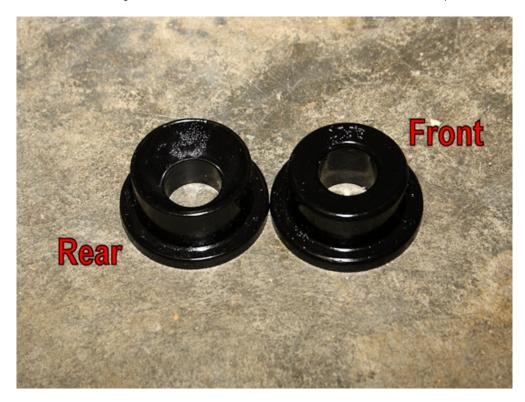
13. Get familiar with how the various parts fit together before you grease and install them. The rear of the arms will use the polyurethane bushing balls nestled between the curved rear bushings. A long sleeve passes through all of the components. The fronts of the arms use the shorter steel sleeve and the flat-faced bushings. When installed, the bushings will be pushed together, but I've left them separated for clarity purposes in the picture below.
