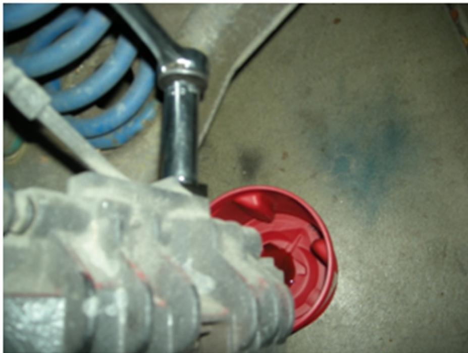
4. Use the line wrenches to loosen and remove the soft brake line from the hard line. Some brake fluid will run out; have a couple of paper towels ready to catch it.
