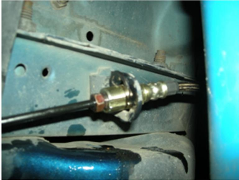
9. Install the bolt with a crush washer on either side of the brake line back onto the caliper.
