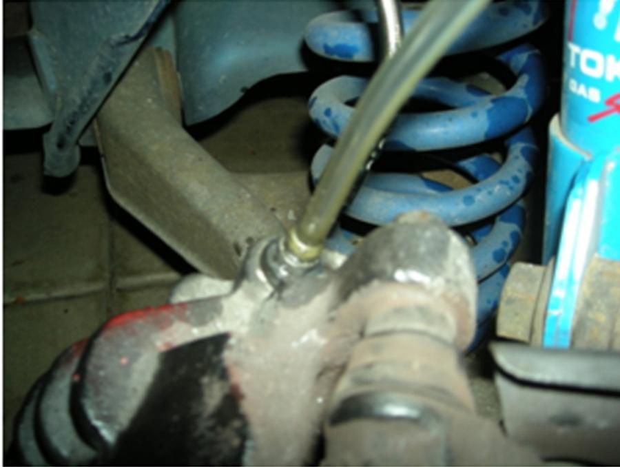
2. Loosen the brake bleeder using a 10mm wrench. Loosen it about a turn and a half. If you are using a brake bleeder kit then hold the bottle somewhere above the caliper and have a friend sit in the car and slowly pump the brake. Watch the fluid coming out of the caliper. There will probably be some air bubbles. When the fluid runs smoothly out of the caliper with NO air bubble then you can tighten the bleeder screw.
