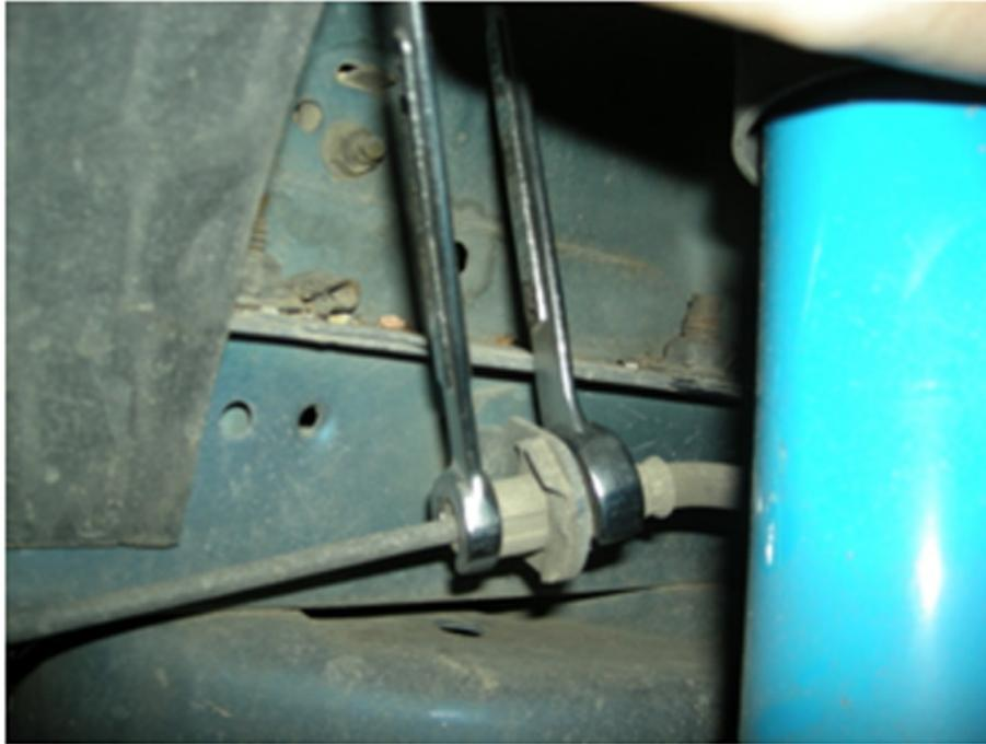
5. Use the pliers to pull the retaining pin off of the old soft brake line. It is fairly easy because there is a lip to grab onto. The brake line is now free and you can set it aside.
