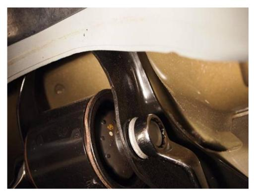
4. Using your 18mm socket loosen and remove the two bolts that hold the Upper Control Arm mount. Pictured below is just one of the bolts.
