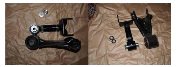
7. Install the J&M arm into the mount. Place the two bushings in the kit on the outside of the UCA mount holes. These are stepped washers that help correct the size of the holes in the mount. When installed correctly the control arm will not move. Loosely tighten the Upper Control Arm bolts, the one on the mount and the other on the differential. From underneath the car tighten the two UCA mount bolts to 85 ft-lbs. Climb inside the car and tighten the last UCA mount bolt to 129 ft-lbs.
