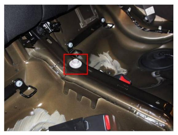
6. After loosening the bolt from inside the car get back underneath the car. You should now be able to remove the bolt holding the Upper Control Arm. In the pictures below you will see a comparison of the stock arm and J&M arm. I found that the J&M UCA came in the same length as the stock UCA and did not need to be adjusted.
