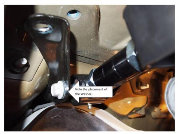
8. After the mount has been tightened down. Load the suspension by raising the car and placing onto jack stands. Tighten the UCA bolts to 129 ft-lbs. You will find that the flag bolt that connects the UCA to the differential will spin because there is no longer an edge for it to catch on to. Use the 18mm wrench to keep the bolt from spinning as you tighten it down. You're done!
