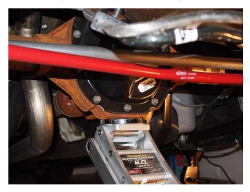
2. Use the 18mm deep socket to remove the nut that connects the stock upper control arm to the rear differential. I found it helpful to raise the differential slightly with the jack to remove the bolt.
