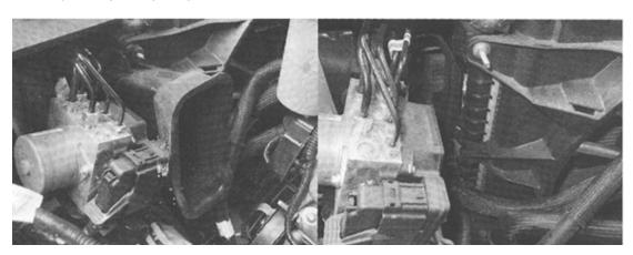
4. Remove the grommet from the stock air inlet removed in step 4 and insert it into the hole in the JLT heat shield and run MAF wire harness along frame rail positioning the plug at the upper right side of radiator.
