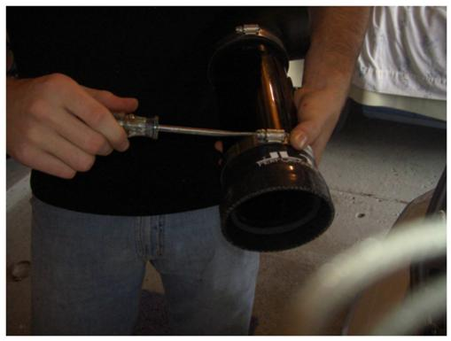
11. Fit the new metal mass air flow sensor housing into the silicon reducer so that the letters "JLT" can be read normally (without turning the intake around) and the slit for the MAFS is again, aligned with the opening of the elbow!! Secure the connection with another clamp.
