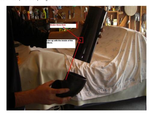
Slide a small metal clamp around the opposite end of the tube and place the black silicon reducer over that end. You should only push the silicon reducer so far so that the black tube ends where the reducer gets wider.
