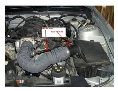
2. All of this stuff must be taken out of the car. First things first, locate the single bolt holding your factory airbox in place and remove the bolt with a 10mm socket wrench. (extension recommended)
