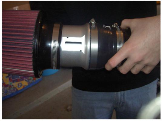
13. After the assembly of your new JLT intake is done, go ahead and take your stock airbox out and put in your supplied heat shield. Using the old stock airbox bolt and your 10 mm socket wrench bolt in the heat shield. Using the supplied zip ties, secure the free end of the heat shield to the round hole in the front of your engine bay. Place your JLT in. put a new clamp over the elbow, and attach it to your throttle body. Again, using a flathead screwdriver, tighten that connection.
