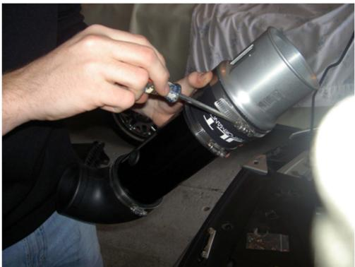
12. Affix the new filter on the other end of the MAFS housing making sure you have enough room to re-insert the MAFS. Secure the connection with another clamp.
