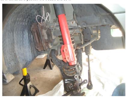
7. **Important:** Now SLOWLY lower the jack, making sure the spindle and control arm lowers as the jack is lowering. You will hear a loud POP! as the strut lowers, this is the sway bar coming off of the sway bar end. Make sure the jack and control arm lower **together!!** Now with all the components hanging down, use a prybar and pull the spring out (you might need to press down on the A-arm with your foot a bit, its ok).
