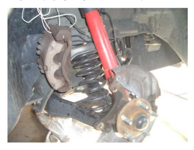
3. Next, remove the brake hoses from the small bracket behind the strut. Removing them from the bracket will give the hose some slack for when you disconnect the strut. You do not want to bend or twist these lines, so be careful, and let them hang down. You may be able to go on without this step if your very careful.
