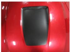
Vinyl that needs to conform to curves of the hood can be pressed into place with your hands or if need be the use of a hair dryer to help conform to the shape of the car. Also when tucking vinyl around the edges of the car. **Do not over heat it will shrivel or wrin-kle.**
