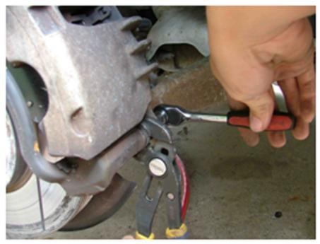
7. Remove the caliper by sliding it out and away from the rotor. This may require prying it out with a large screwdriver. Be sure not to let the caliper hang by its brake line. You can set the caliper just behind the rotor to prevent damaging the brake line.
