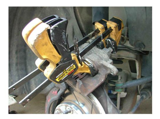
13. Slide the caliper back over the brake pads and screw in the bolts.
