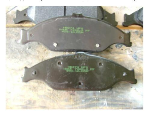
10. Spread grease over areas shown below. This should include any places where the brake pad contacts the caliper and the caliper bracket.
