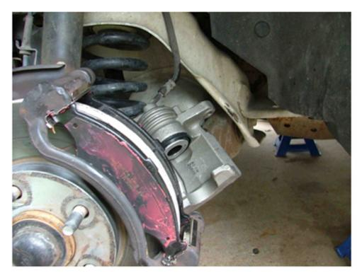
12. Compress the pistons back into the caliper as shown below. Although a c-clamp is best to use, any clamp should work.
