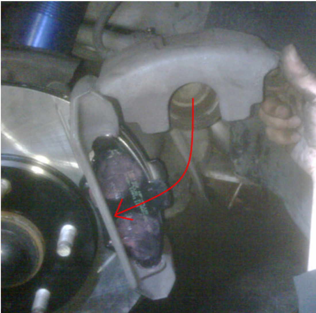
Brake caliper swings down on upper dowel.
