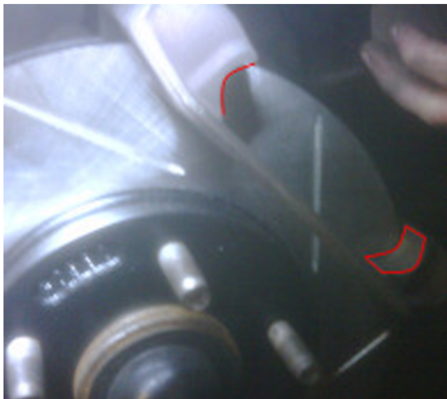
Pad/caliper retainer on rotor. The pad seats to be greased are circled in red.
