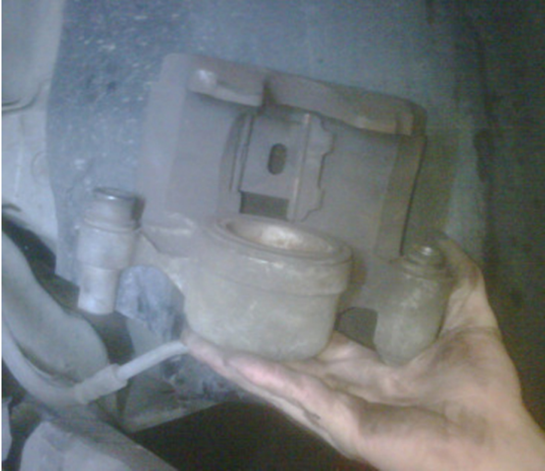
Compressed piston. Notice the piston is flush with the cylinder wall.
