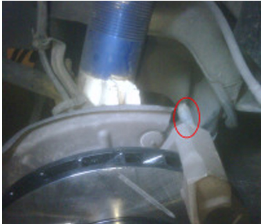
Pad/caliper retainer on rotor. The caliper dowel to be lubricated is circled in red.
