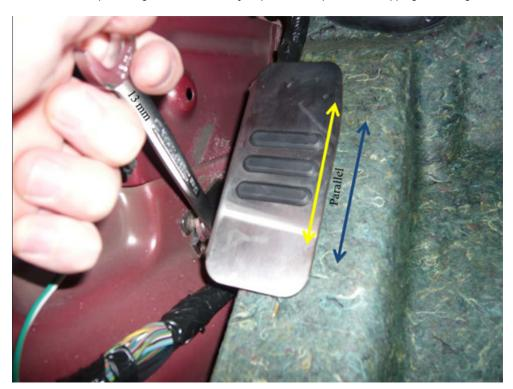
8. Push the carpet back under the pedal, making sure that the carpet is lying flat against the floor, and that there are no 'bubbles' in the carpet.
