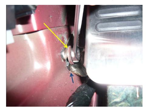
6. Note: If the pedal does not sit almost flush with the existing footrest area, use a grinder or file to remove the sharp corner of the pedal (blue arrow) to give it sufficient clearance for the floor pan. \*\*There does need to be enough space for the carpet to slide back under, so don't get carried away!\*\* If you do grind down the pedal, do it in small amounts and retest the fit every time.
