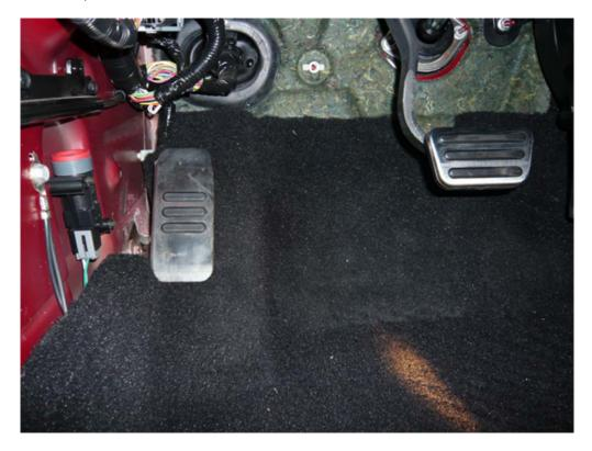
9. Replace the plastic cover and make sure door sill is tightly back in place. If the panel is loose, double check the clips to make sure they are lined up properly. It might be a good idea to leave the plastic screw out until you are completely satisfied with the installation of the pedal.
