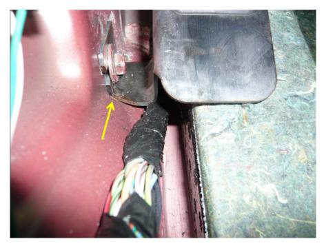
As you can see, the bottom of the pedal may scrape the floor pan, making the install more difficult.
