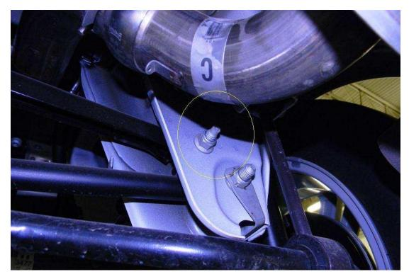
Slide the muffler towards the <u>front</u> of the car; insert the two (2) rear hangers into the rear grommets. Slide the muffler to the <u>rear</u> of the car to fully support the new exhaust system. It may be necessary to manually adjust the new FRPP exhaust hangers to fully insert them into the rubber grommets. Adjust as needed, being careful not to break loose the new welds.
