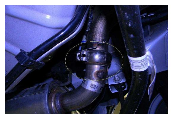
Gently slide the old stock exhaust system towards the front of the car. The stock exhaust pipe is retained. Do not remove.
