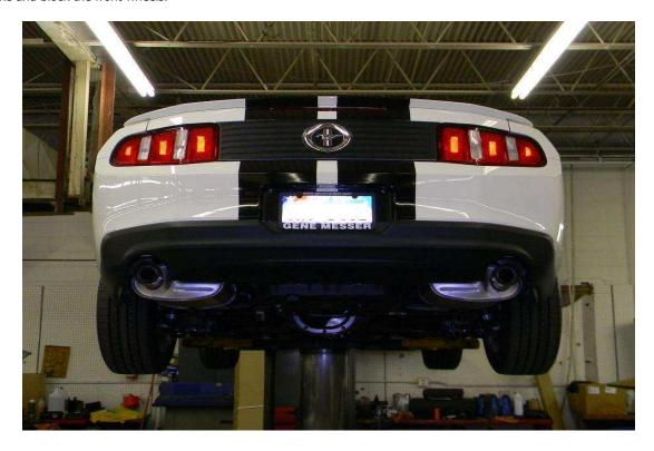
Position yourself under the car to access the old stock exhaust system, inspect the work area and position your tools for easy access.
