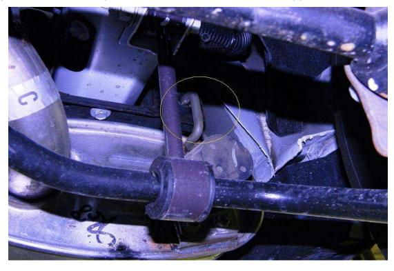
Remove the coupler from the old stock exhaust. You will need to cut the factory mounting tab to remove the coupler. You can use a Dremel tool or other cutter. It is not necessary to weld the coupler onto the new FRPP muffler system.
