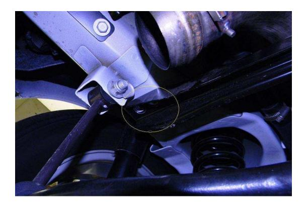
The new FRPP exhaust is ready to install. Place one (1) coupler onto each side of the new exhaust mufflers. Use something soft to cover the new exhaust tips to prevent scratches during the installation. Insert the front exhaust hanger into the rubber grommet, supporting the weight of the new FRPP exhaust system.
