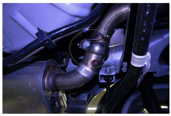
Now remove the rear exhaust hangers from the rear hanger grommets.
