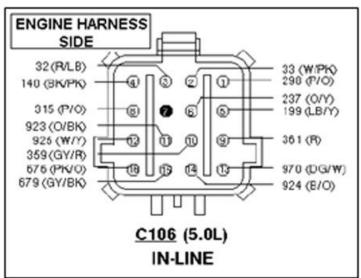
On 4.6L applications, circuit 361 may be located in cavity 5
