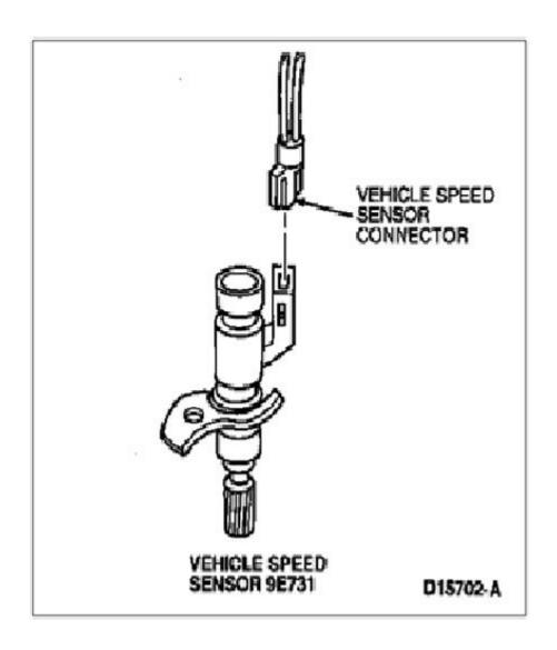
2. Identify the VSS (+) signal output wire. The wire colors are typically GRAY/BLACK on the VSS (+) signal side, and PINK/ORANGE on the VSS (-) return side. Remove the harness wrap to expose approximately 6 inches of the VSS wire leads, and cut the GRAY/BLACK signal wire, insuring that there is enough wire remaining on each side to splice in the wires coming from Speed-Dial.
