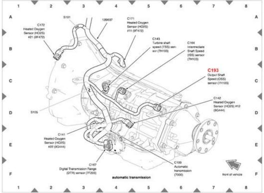
2. Identify the signal output wire. The wire colors are typically BLUE/YELLOW on the OSS (+) signal side, and GRAY/RED on the OSS (-) return side. Remove the harness wrap to expose approximately 6 inches of the OSS wire leads, and cut the BLUE/YELLOW signal wire, insuring that there is enough wire remaining on each side to splice in the wires coming from Speed-Dial.
