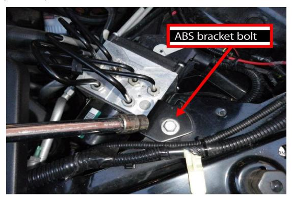
9. Install the provided stud in this location. You will need a 15mm wrench for this. A 15mm deep socket speeds up the install.
