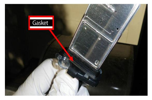
7. Install MAF into new airbox with the screws provided. They already have thread locker on them.
