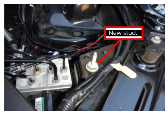
10. Place new CAI airbox in this location. Carefully align the stud and the two rubber bumpers on the bottom into the respective holes. Everything should line up with minimal force. Once in place, install the provided nut on the stud. 10mm deep socket is helpful here. Also, install your existing 10mm airbox retaining bolt.
