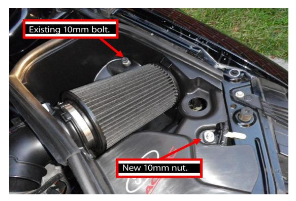
11. Install new clean air tube. Be sure it is fully seated on the airbox tube and throttle body. Tighten the hose clamps.
