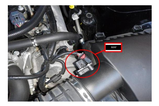
3. Disconnect the PCV line. There is a green tab that must be pulled out to release the tube. The green tab is on the bottom of the fitting. You can see a ridge on the PCV tube coming from the clean air tube. The green tab has to clear this
