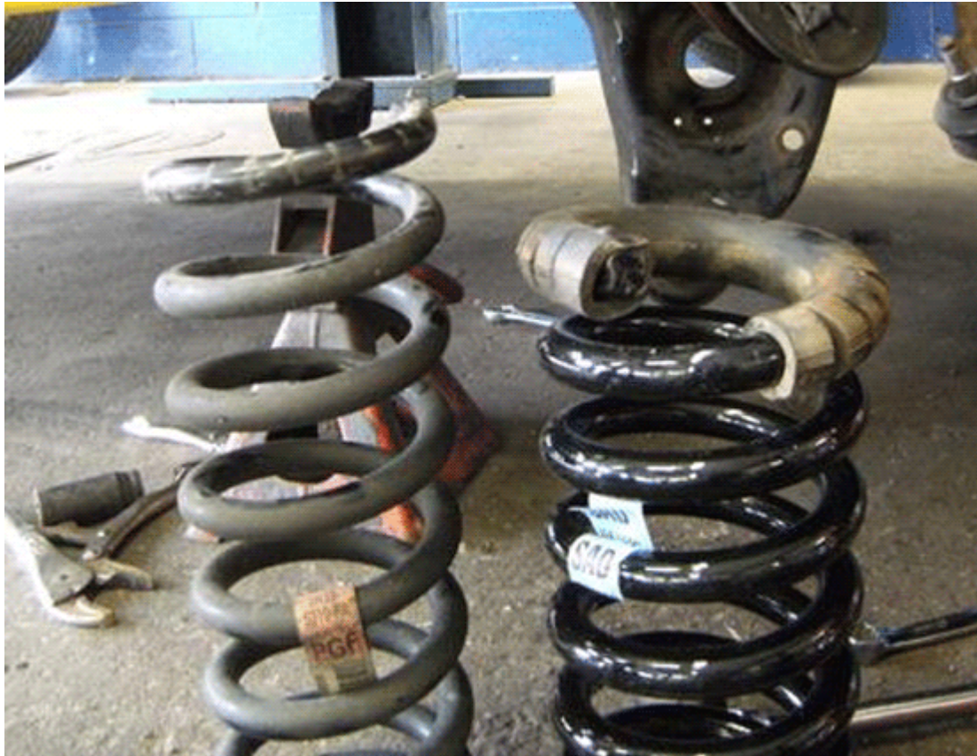
C- Spring vs. Stock Spring. Notice thicker coils and much shorter height
