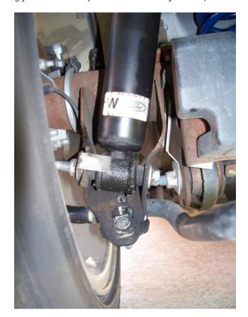
18. Remove brake line bracket on both sides of the car.
