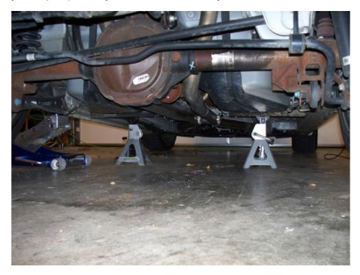
16. Unbolt your rear anti-rollbar clamps on both sides of your car and flip your rollbar to the rear of your car out of the way.
