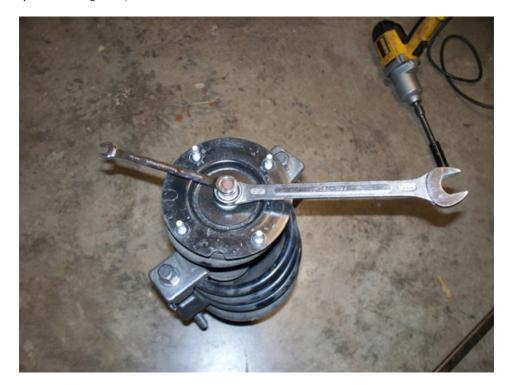
12. Note: you will find a black rubber coil protector/isolator on your stock front spring and you will need to remove this and place it on the bottom of your new Ford Racing springs. On your new Ford Racing springs you will find a clear plastic protector about two coils up I left this alone and installed the OEM black isolator below this.
