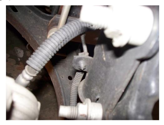
6. You will need to break lose the upper front anti-rollbar link from the strut housing. (Using 18mm deep well socket.)
