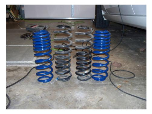
20. New Ford Racing Mustang K-Springs installed. Work was done on 2007 Mustang GT. Any time when lowering your car you will need to have your alignment check.
