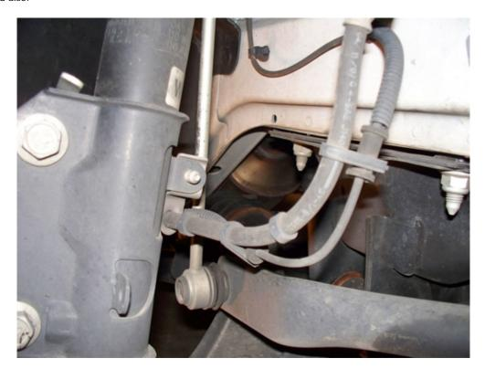
5. Now remove the ABS electrical wire support plastic one way clamp. (Needle nose pliers will help a lot when removing this.)
