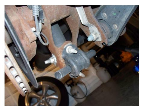
17. Remove the bolt holding your rear shock in place on both sides of your car. (Use 15mm deep well socket.)
