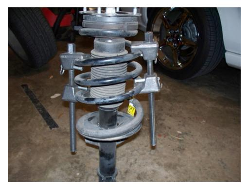
11. Now that the spring is compressed use a 22mm open end wrench to break the nut lose then you will need a 10mm open end wrench as shown in picture to remove the nut from the strut assembly. Once you have removed the nut pull the strut bearing cap off. (If the bearing cap does come apart don't worry it's not a big deal just place the bearings back into and put it back together.)
