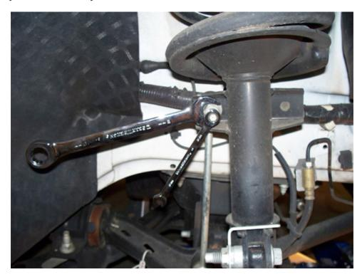
8. Now remove the two lower strut bolts and nuts from the spindle. (Use 18mm deep well socket with 6 inch extension.) Support the brake assembly with some wire or rope to lessen the strain on the brake lines on both sides.
