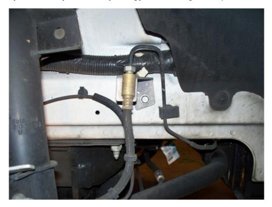
4. There is another 10mm bolt holding the brake line in place that is located behind the front strut the need to be removed also.
