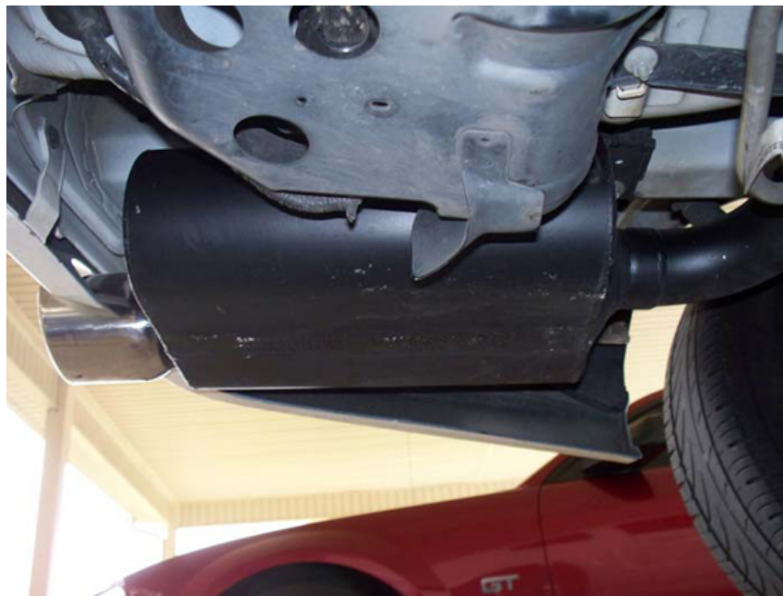
New Mufflers Installed
