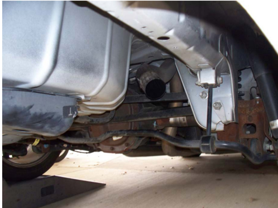
After Removal of Mufflers
