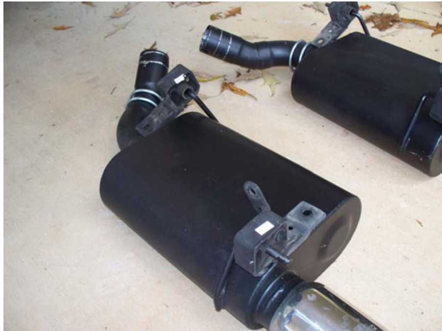
Rubber Isolators Placed on New Mufflers
