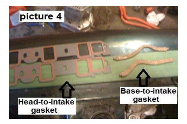
7. Now put the intake in place. Be careful to not move the <u>gasket</u> when you do this. I personally recommend to remove the distributor. You will see in your new or old intake bolts that they have 4 different bolts compared to the others (little more wide, if you don't have this bolt just be careful to align the intake with the head) put these bolts (or if you don't have it just 4 normal bolts) in the corner of the intake then put it in place then screw all bolts with hand-force.
