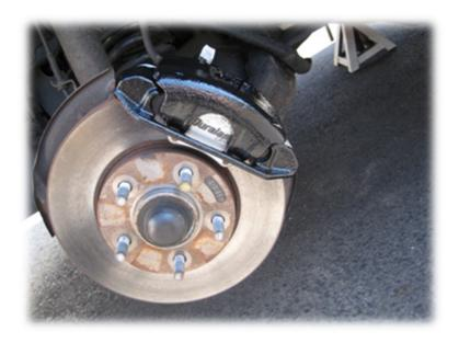
9. The paint will be dry to the touch within 1 hour. After the paint is dry, you can then reinstall your wheels, finger tighten your lug nuts in the star pattern, raise the car slightly with the jack so that the jack stands can be removed and SLOWLY lower the car back to the ground. Finish by securely tightening the lug nuts with the star wrench in the same start pattern as before.
