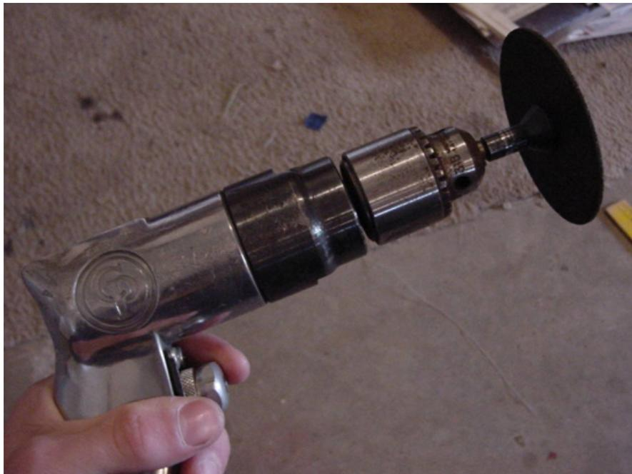
5. Start cutting the exhaust pipe with the cutting tool as pictured above and if you work slowly but surely the pipe will cut. I used a pneumatic air drill but a regular drill works just as well. Metal cutting wheels can be purchased at any hardware store. I believe a pack of five cutting wheels costs about \$6.00. It just takes a little time and patience.
