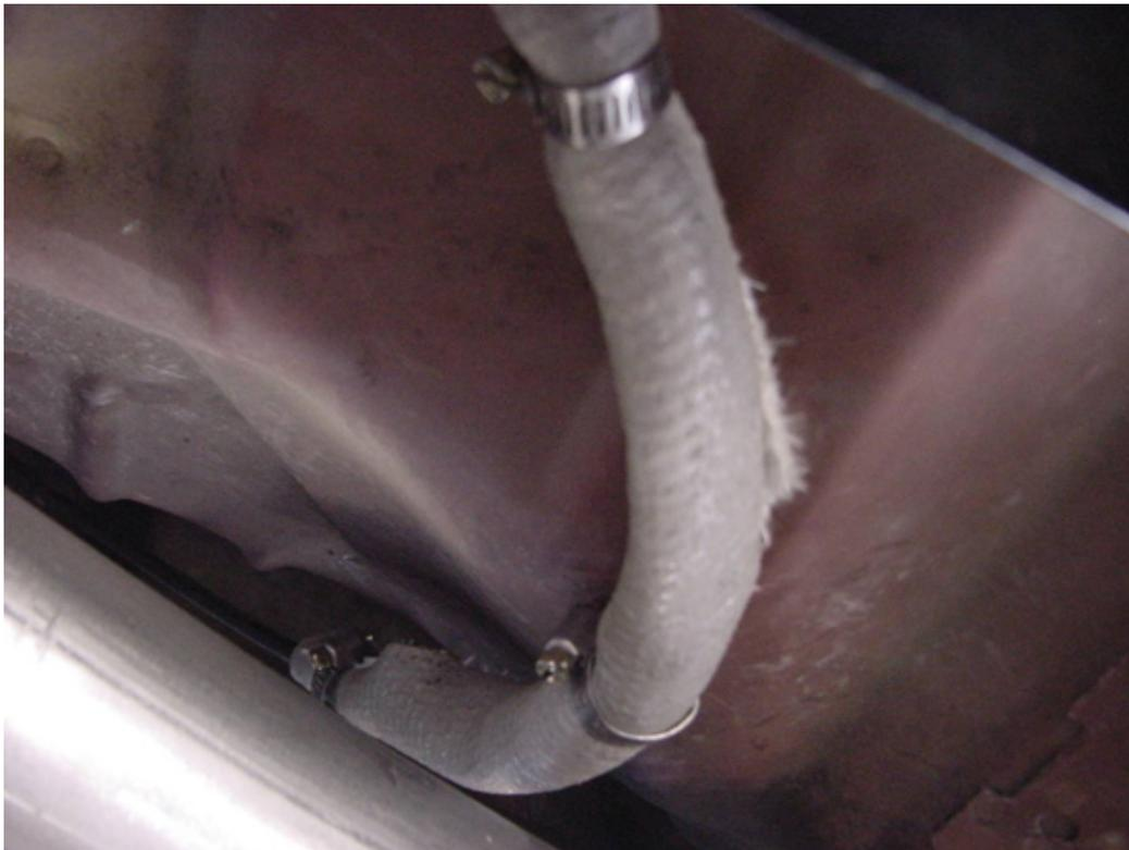
9. After looking under the car, you can see that there is a brake line on the driver's side of the car that is very close to the adapter. The brake shield is designed to go over this brake line so that it shields the line from the heat. Start by taking the heat shield tubing and make a cut in one side of the shield from one end to the other. After this is completed, it will just slide over the line and use the three clamps to hold it in place so that it will not slide down the brake line.
