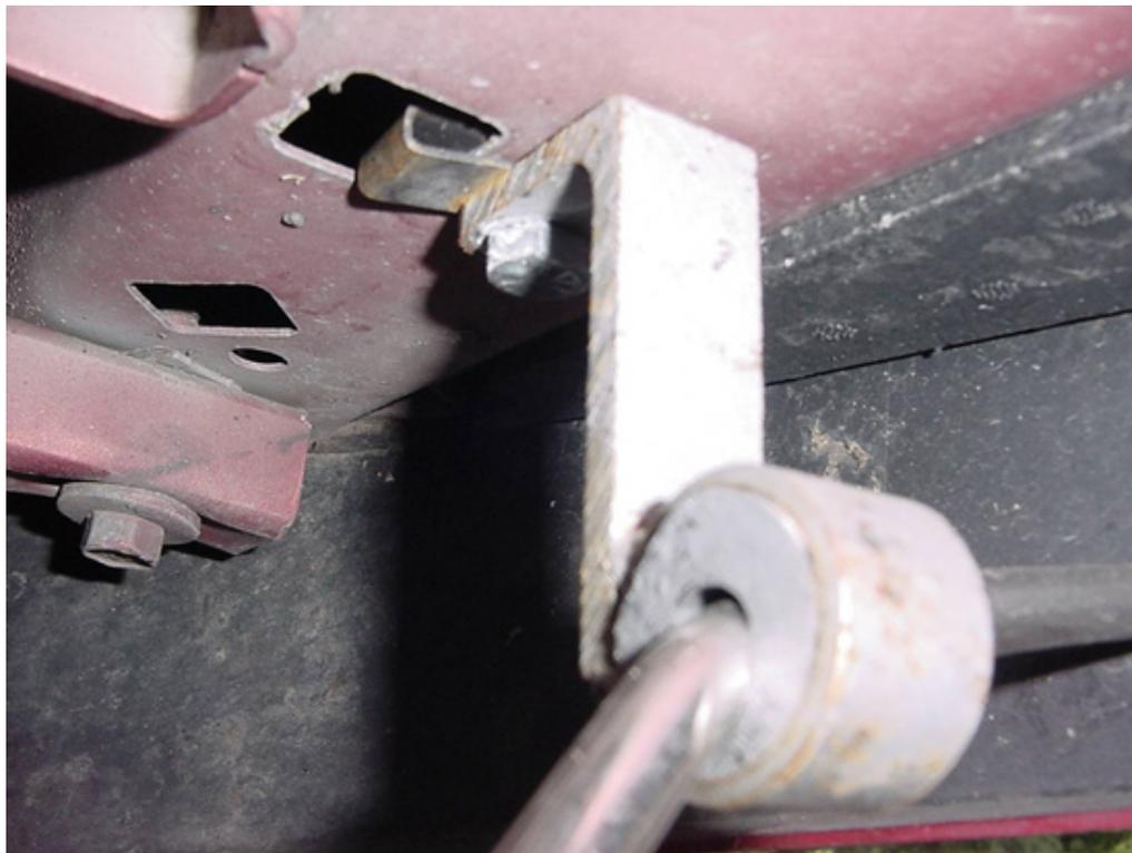
13. Below is an image of what not to do when completing this installation. Make sure that the U bolts holding the old pipes onto the adapter are very tight. I did not tighten them down enough and the adapter slipped off of the passenger's side of the car. Unfortunately, the adapter kit would not fit back over the pipe so I needed to go to a local auto shop and purchase a coupling that would hold the adapter to the original pipe on the car.
