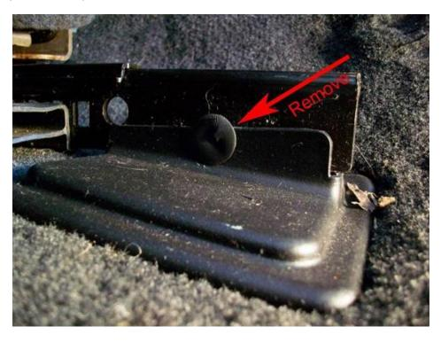
6. Once the plastic keepers are removed, pull up on the plastic covers and unsnap them from the sliders. Underneath are the remaining bolts holding the seats to the floor. These bolts will take much more persuasion to break free than the nuts did in the front.
