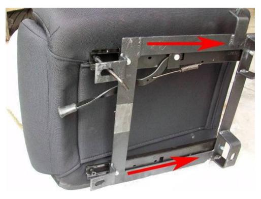
5. Slide the bracket to the forward position and align the holes in the back. Reinstall the 6mm bolts and tighten them down.
