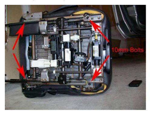
13. Disconnect the lumbar power cable and pull away the metal sliders.
