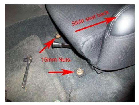
11. Slide the seat to the forward position and line up back holes. Before installing bolts, put a small bead of thread lock around the middle of each one. This will prevent moisture from building up underneath the new seats. Tighten bolts to about 40 ft/lbs.
