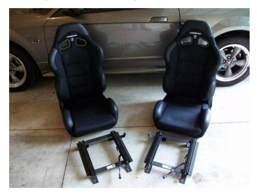
3. Unscrew the four bolts that come on the bottom of your new seats using a 6mm hex wrench.
