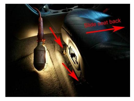
3. Using your 15mm wrench, remove the two nuts holding each seat to the floor. These studs are stationary, DO NOT attempt to remove them.
