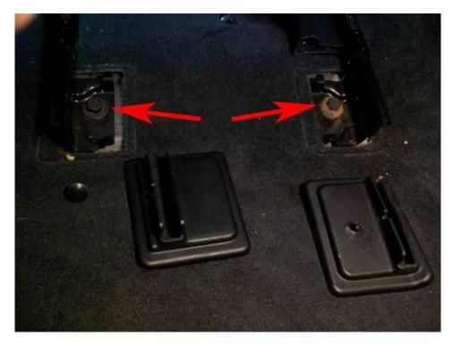
7. Because the bolts go through the floorboard, they are exposed to the elements and can become corroded. It is recommended that you apply rust penetrant to the studs sticking through the floorboard to ease the removal process.
