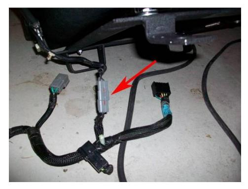
9. Before bolting your new seats down, tilt the driver seat backwards and reconnect the wire harness back into its original connector. Feel free to use tape or zip ties to manage the extra wires.
