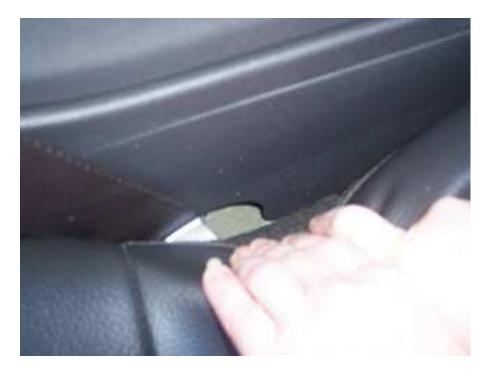
4. Once hooked under, use the velcro strip to cinch the tie-down strap tightly so that there is no movement in the windstop.
