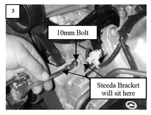
4. You can now mount the Steeda Idler Bracket with the supplied hardware. Position the bracket in the location of the two bolts you removed on the timing cover, see picture #3. Use the supplied 10mm bolt and washer to bolt the bracket down to the timing cover, see picture #4. Then use the supplied 13mm bolt and washer to bolt the brackets to the timing cover horizontally.
