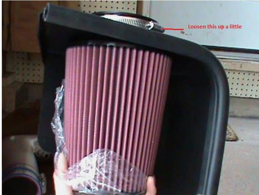
5. Set the MAF housing and air filter aside. Take the C&L intake tube and loosen up the four clamps. A standard screwdriver works best for this.
