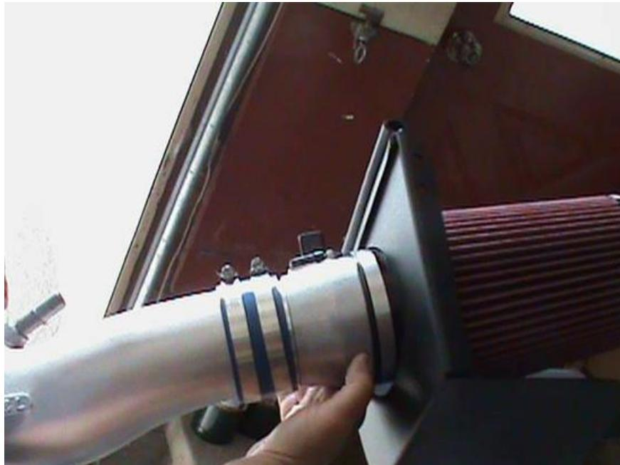
7. Move the two clamps back to where they originally were and tighten down the two clamps with the standards screw driver. You should now have what the picture above shows.
