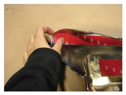
3. Once the backing tape is removed, position the covers on the mirrors to insure they are aligned properly. Take care not to press down on the trim during this step.
