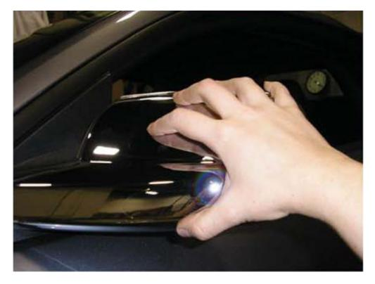
4. When you feel you have successfully lined the covers up with the form of the mirror, press firmly along the entire surface of the covers to ensure a complete and sturdy bond is made with your mirror.
