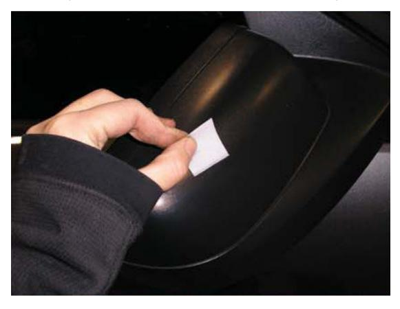
2. Before applying the covers, make sure all of the backing is completely removed from the 3M bonding tape.
