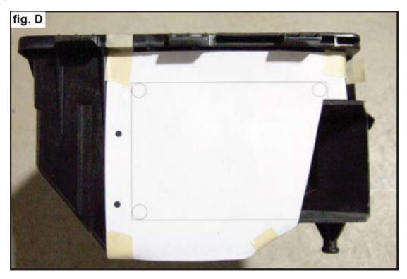
6. After the ram air box conversion component has been painted black, install it to the factory air box. Use two small black Phillips screws in the pre-drilled holes in the front of the air box. Drill two 1/8" holes in the back of the air box and install two more small black Phillips screws as shown in Fig. E.
