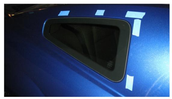
4. Cut strips of 3M tape to fit on underside of window scoop along the edges. Press down firmly. Remove red tape backing.
