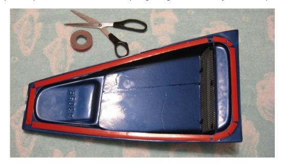
Align window scoop in place over window without actually touching it to the car. Align the top edge and the front top corner of the scoop to the painter's tape. Press firmly on top corner and on all edges. Apply pressure and hold in place for 2 minutes.
