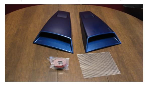
4. Before installing, hold the window scoop up to the Quarter Window to see positioning. The straight edge of the window scoop should be at the top, to follow the line of the car. The drain hole should be near bottom corner. Window should be covered completely by the window scoop.
