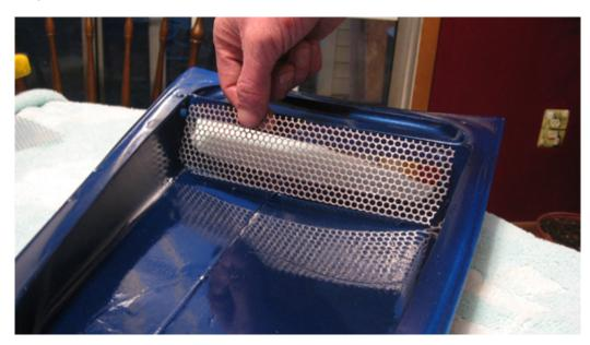
4. There are 5 screws for each window scoop. Insert each through holes in screen and tighten with Philips head screwdriver. (If you have trouble aligning the fourth screw, you may need to clip just the center piece of screen covering that hole so the screw will fit in). Tighten screws flush so that the head of the screws hold the screen in place. Repeat process for second window scoop.
