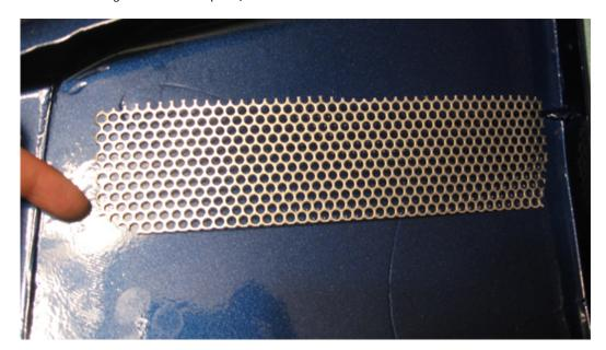
3. Position the screen, again, into the window scoop and check to make sure that the screw holes in the window scoop line up with holes in the screen. If they do not line up, then you can trim it again to match. Then cut the rest of the screen to size in a straight line.
