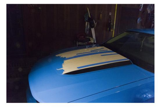
3. Measure and mark the centerline of the hood. Be extra careful here because this is where the CDC template will line up.
