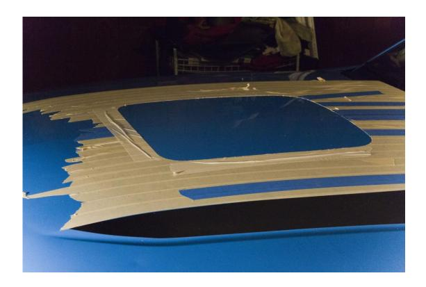
6. Cut hood along the template cut out. Make sure to tape over the cut line if the hood starts to vibrate too much.
