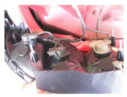
6. After you have placed all the light bulbs into your new taillights, remember to place the wire holder into the small holding socket located below and between the two outside lights on the back of the taillight. This will hold your wiring in place.
