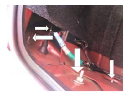
4. After removing the nuts, set them off the side for installing your new taillights then proceed to remove the taillight fixture. Removing the taillight can be difficult so you can use a hammer to lightly tap on the back of the bolts and it should come out easily. You can then proceed to remove the light bulbs from the back of the taillight by twisting them out of their sockets.
