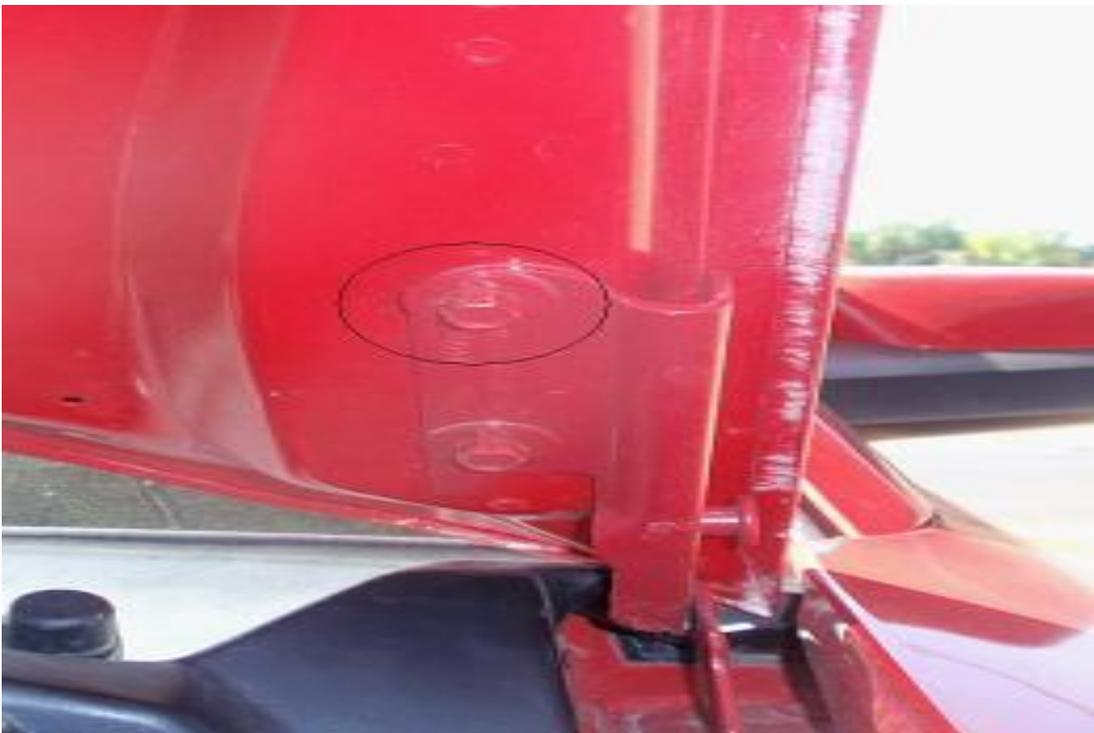
5. Locate the large bracket marked D-U. Now loosen the bottom bolt on the hood hinge just enough to slide the larger bracket between the hinge and the bolt as shown. **DO NOT REMOVE BOTTOM BOLT.** Tighten bottom bolt first and then re-install top bolt to secure bracket. ( Note: Align the top bolt holes before tightening the bottom bolt.)
