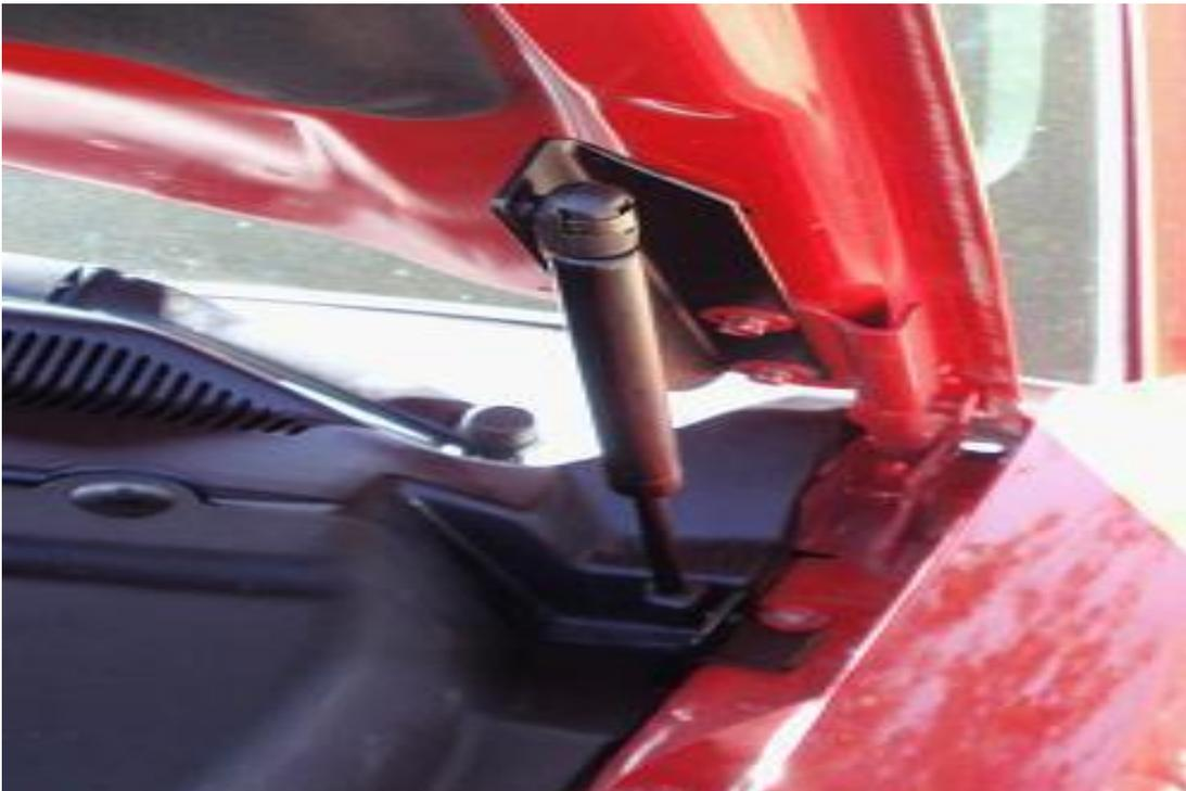
7. Repeat steps 2-6 for passenger side hood strut to complete the installation.
