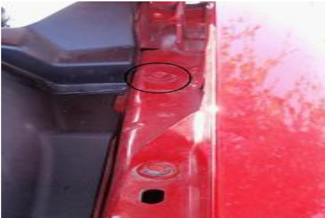
3. Install small bracket marked D-L and tighten using factory fender bolt as shown.
