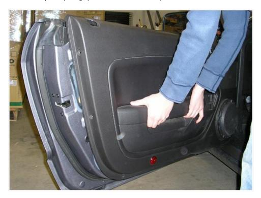
11. In order to remove the door release cable, you will need to remove the door handle assembly. To do this, use a small flathead screwdriver wrapped in a shop towel to pry away the faceplate and/or push from the back of the assembly. There are two clips on the bottom. You will need to use a significant amount of force.
