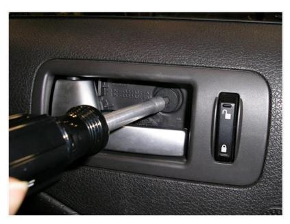
2. Remove the cover from the door pull/armrest area. You may need to use a small jeweler's flathead to pry it forward and away from the main door panel to release it. Remove the T30 Torx screw from behind it.
