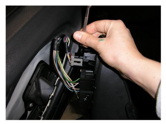
4. You will now have access to the back of the door handle. Using the jeweler's flathead wrapped in a shop cloth, or a hook tool, remove the plastic panel front around the door handle. To release the clip that is holding the panel in place, you will want to pry from the lower inner side of the panel. Putting the door handle in the open position will also assist in its removal.
