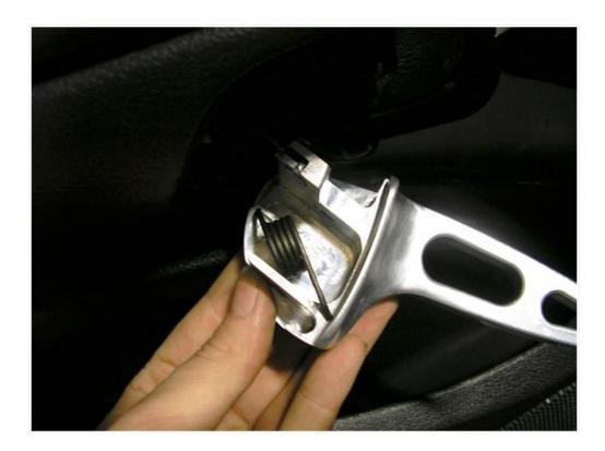
9. Using the supplied hardware, reinstall the handle. You will probably need to use your Phillips Head screwdriver to push the hardware through. Secure with the nylock nut. Nut should be tight, but no so tight as to bind the handle to the assembly.
