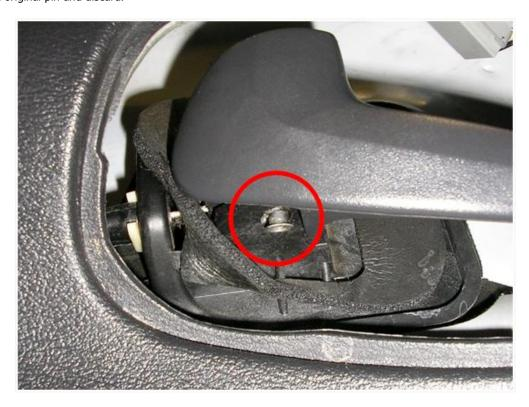
6. Before removing the old handle, not the direction and orientation of the old spring, which will be reused. Remove the spring, and make sure to put it somewhere you won't lose it.
