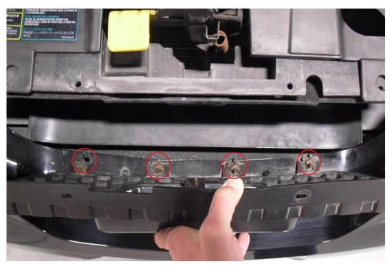
3. Remove two of the threaded clips from your factory honeycomb grille and place them on the lower mounting brackets of the billet replacement grille.
