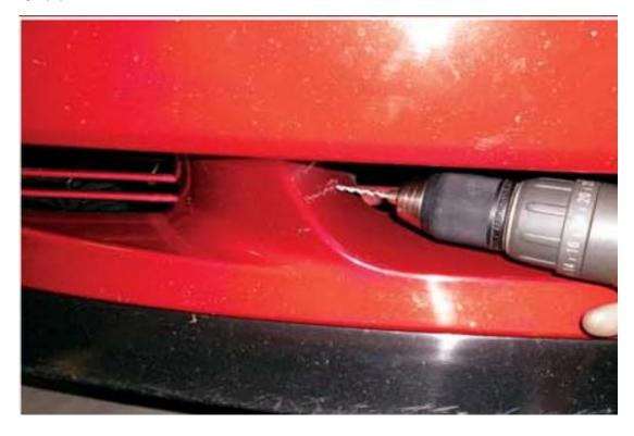
5. DO NOT DRILL all the way through your lower grille's side opening-you only need to drill through the first panel.
