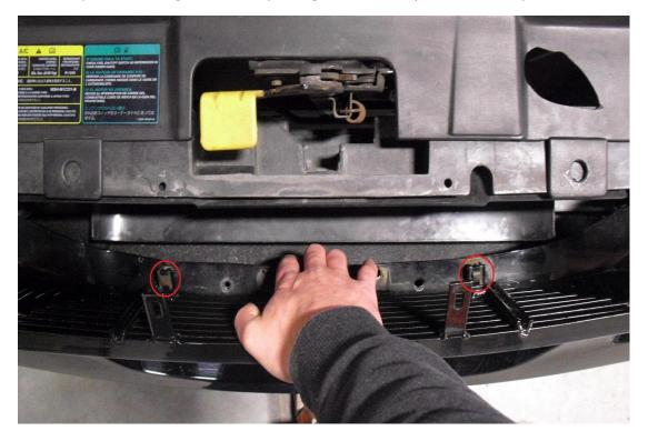
5. Attach the upper grille using the factory plastic retaining pins that you removed in Step 1 to complete the installation of your upper billet replacement grille.
