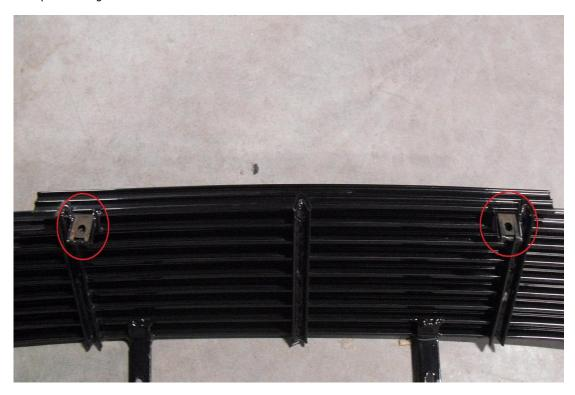
4. Attach the lower part of the billet grille to the bumper using two of the bolts you removed in Step 2.
