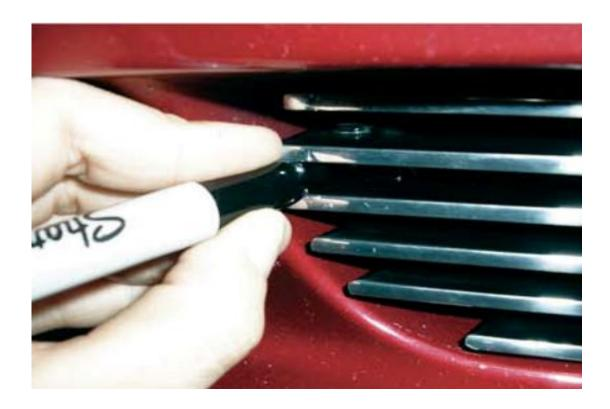
4. Remove the grille. Using your marked locations, drill a hole in each side of the lower grille. You will need to sue a 3/16" for this, however, you may minimize chipping by drilling a smaller pilot hole before drilling with the larger bit (or by using masking tape).
