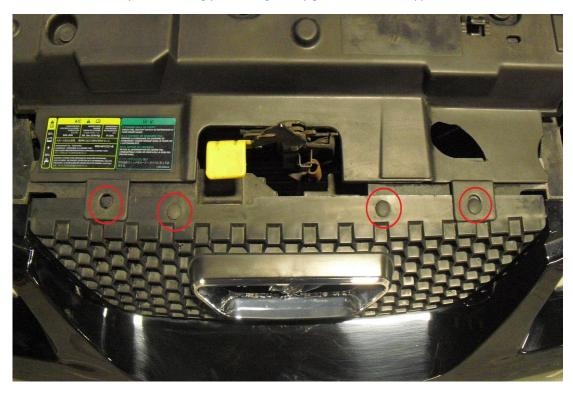
2. Once the upper part of the grille is free, carefully pry the grille back and use a 7mm socket or wrench to remove the four bolts holding the lower part of the grille to the bumper.
